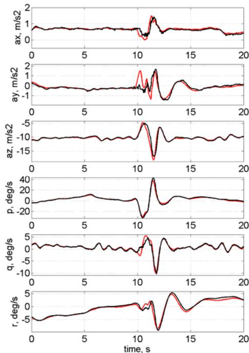
Fig. 19 Do128 lateral wake fly-through: simulation output with wing and fuselage drag modelling (—) compared to flight test data (—)
