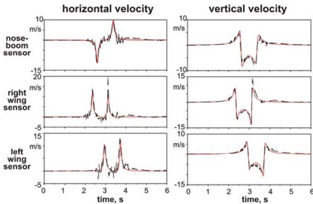
Fig.10b Lateral wake fly-through with high quality boom mounted 5-hole probes: wake model velocities (—), flight test measured (—)
