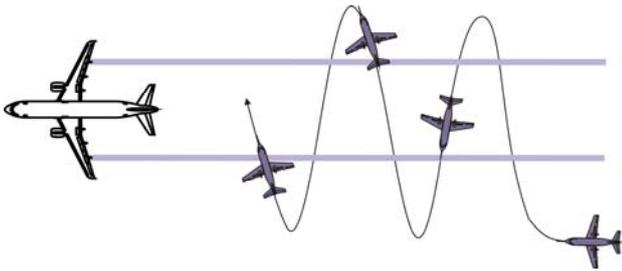
Fig. 2 Flight test scenario for wake determination and encounter model validation; in practice the lateral encounter angles are somewhat smaller ( $25^\circ$  maximum)
