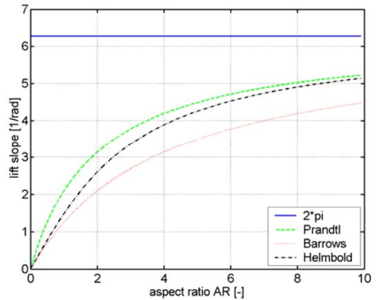
Fig.14 Different approximations for lift curve slope depending on aspect ratio AR
