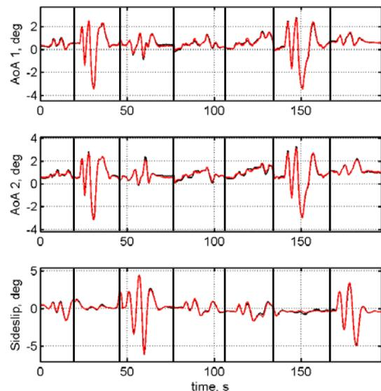
Fig. 7 Calibration results of AoA left/right and sideslip on a MEDIUM size transport aircraft in undisturbed air, model output (—); measured (—●—)
