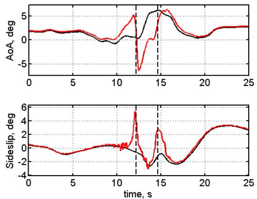
Fig. 9 Lateral wake fly-through: reconstructed inertial AoA/sideslip *without* local wake induced flow angles (—), flight test measured (—)
