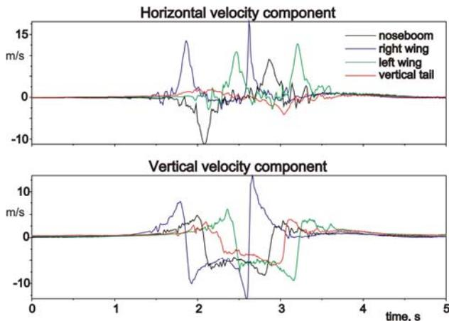
Fig. 6 High quality 100 Hz flow probe measurements of the Do128 aircraft during a lateral wake encounter
