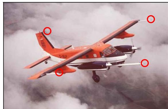
Fig. 5 Do128 wake encounter aircraft of Technical University Braunschweig, **O**= positions of flow probes
