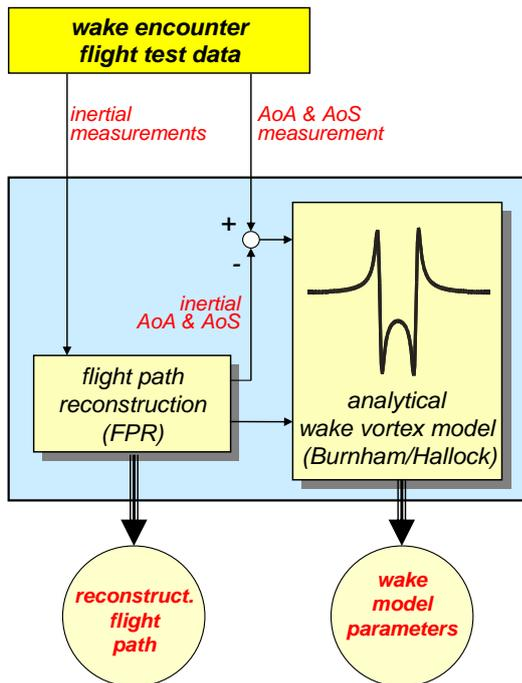
Fig. 8 Principle of wake identification and flight path reconstruction
