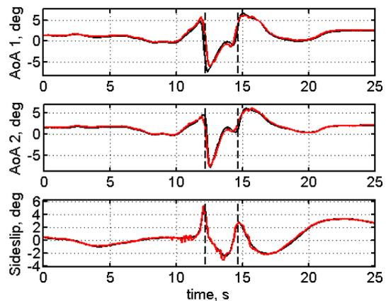
Fig.10a Lateral wake fly-through, fuselage vane equipped aircraft: reconstructed inertial + local wake induced AoA and sideslip (—), flight test measured (—)
