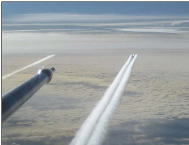
Fig. 4 Wake visualisation by contrails in cruising altitude
