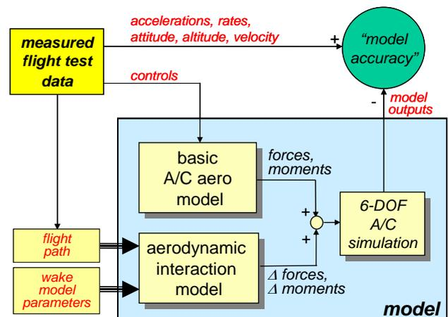
Fig.15 Method to validate wake encounter models from flight test data
