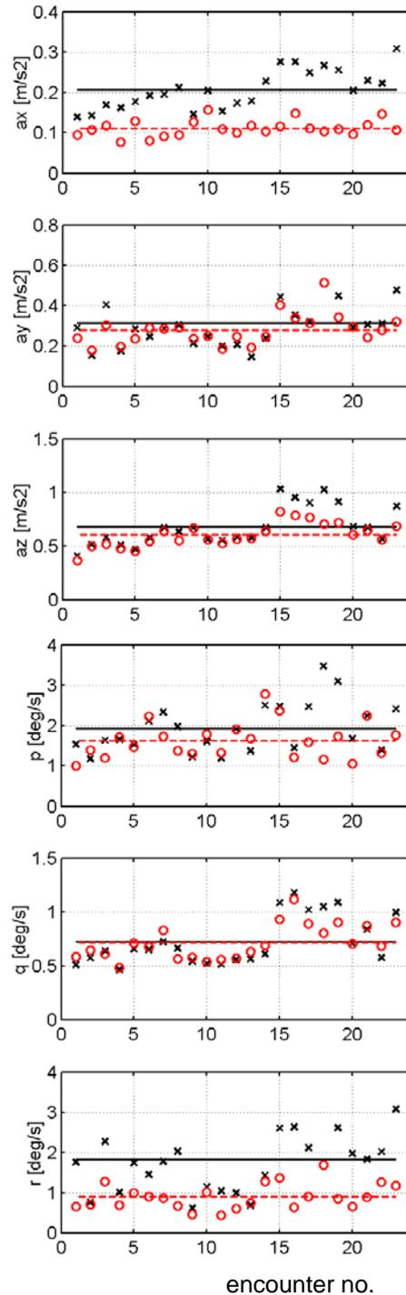
Fig.18 Model improvements for 23 wake encounter simulations: standard deviations of the errors between model outputs and the corresponding flight test data; without (x) and with (o) wing and fuselage drag effects; the lines give the *mean* error standard deviation of all 23 encounters
