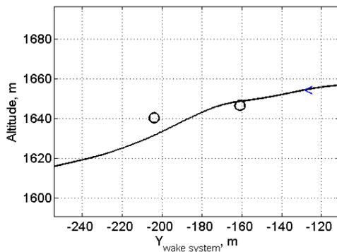
Fig.11 Lateral wake fly-through: reconstructed wake positions (o) and flight path in the wake axis y/z-plane (—)
