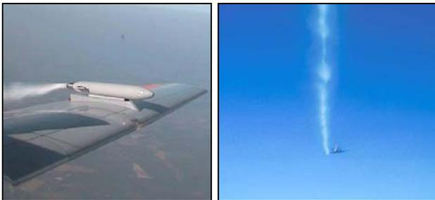
Fig. 3 Wake visualisation by smoke in approach altitude
