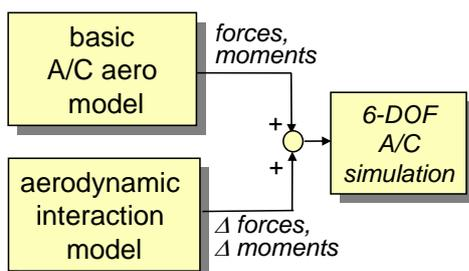
Fig.12 Forces and Moments from basic aero model and wake encounter model
