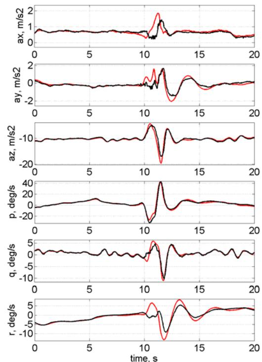
Fig.16 Do128 lateral wake fly-through:
