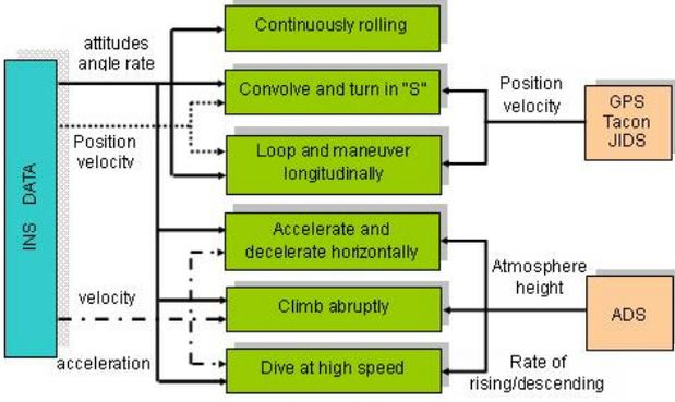
Fig.4 The configuration of functions on navigation flight test data and maneuver flight status
