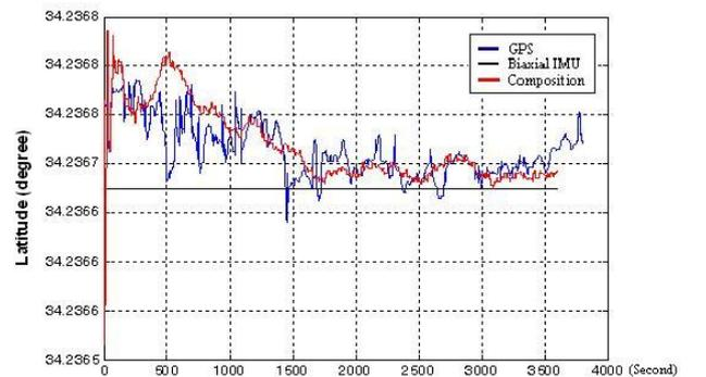
Fig.11 Latitudes of static tests for GPS-Composition-Biaxial IMU
