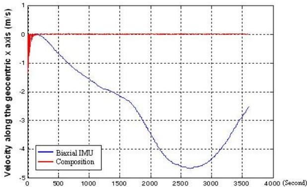
Fig.13 The velocity curves of a composition and biaxial IMU along the geocentric x axis at static condition
