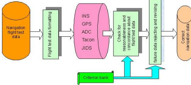
Fig.3 The pre-processing algorithm for navigation flight test data
