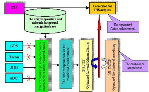
Fig.6 INS-JIDS integrated algorithm frame
