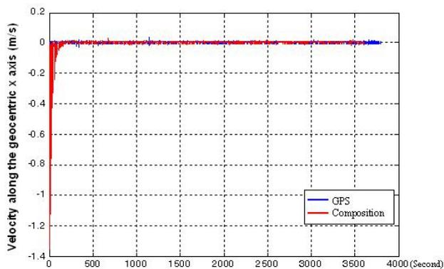
Fig.14 The velocity curves of a composition and GPS along the geocentric x axis at static condition
