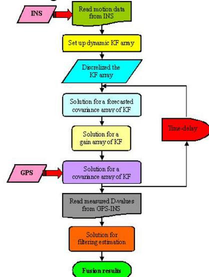
Fig.9 GPS-INS integrated algorithm flow
