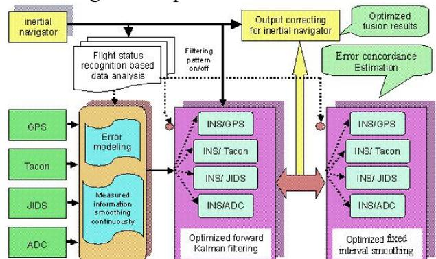
Fig.1 The core of navigation information fusion
