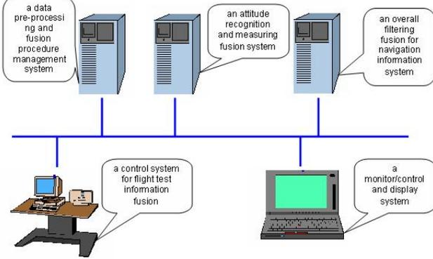
Fig.2 The information fusion processing system based a distributed network configuration
