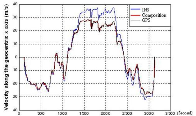
Fig.16 The velocity curves about INS, GPS, and integrated navigation along the geocentric x axis in flight
