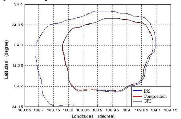
Fig.15 The flight test tracks about INS, GPS, and integrated navigation
