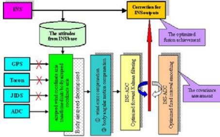
Fig.7 INS-ADC integrated information fusion frame
