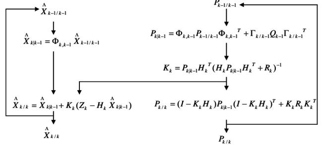
Fig.8 Kalman filtering flow diagram
