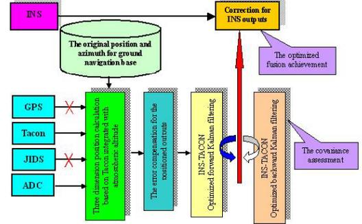
Fig.5 INS/TACON integrated system
