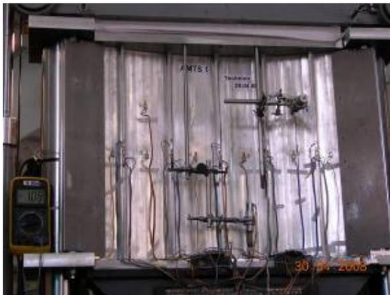
Fig. A3-1. The panel is after buckling (Load  $P_{cr1}=10.6$  Ton). On Picture Load 10.9 ton Laser weld.
