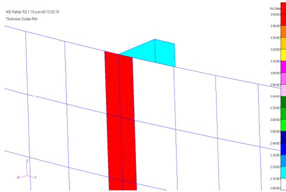
Fig. 3.1 Types of shell's elements categorized by thickness
