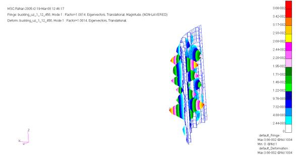
Fig. A1-1 Buckling of the Supported Panel. View in profile (laser weld of stringers).
