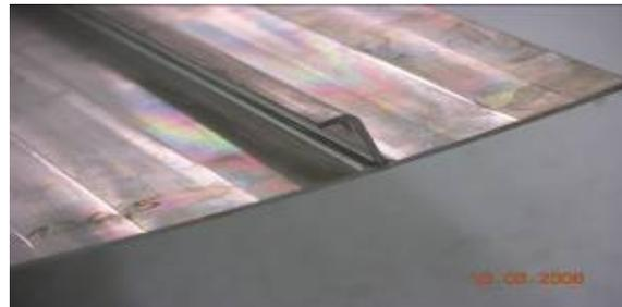
Fig.2.3 Stringer joined by LBW welding.
