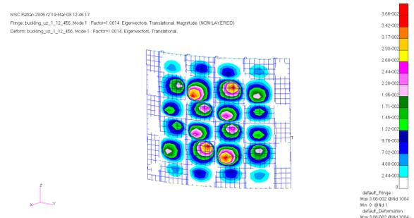
Fig. A1-2. Buckling of the Supported Panel. View in face (laser weld of stringers).
