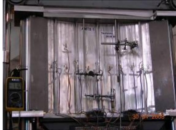
Fig. A3-2. The panel is before plastic state (Load  $P_{cplastic}=11.2$  Ton). On Picture Load 11.0 ton Laser weld.
