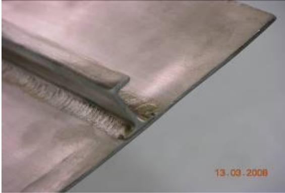
Fig.2.5 Stringer joined by TIG welding.
