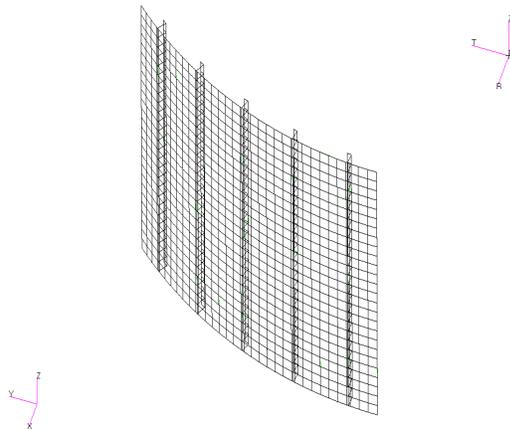
Fig. 3.2 General view of FE model for NASTRAN Code
