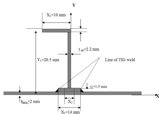
Fig.2.4 The sizes and attachment of a stringer by TIG welding.
