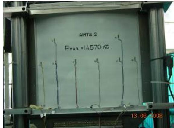
Fig. A2-5 Residual plastic deformations after unloading the panel. Side external. TIG Weld. Irreversible plastic deformations of a skin are visible
