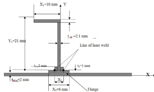
Fig.2.2 The sizes and attachment of a stringer by Laser welding.
