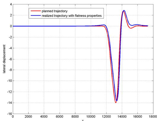
Fig 4.1 Planned and achieved trajectory (lateral displacement)
