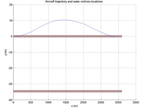
Fig. 2.1: Aircraft optimized trajectory (in red : footprint of the vortices)
