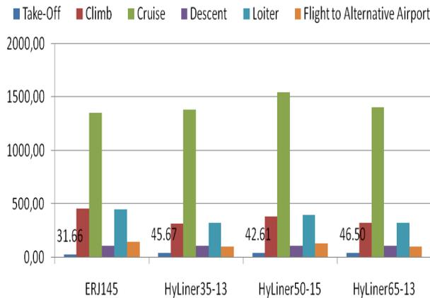
As a result of the ESTOL requirement (Table 1), all presented aircraft have a higher thrust to weight ratio, enabling them to have a faster and shorter climb phase. The climb power depends on the overall overpower. With the higher thrust to weight ratio, the presented configurations are able to climb faster and so to finish the climb phase in a shorter horizontal distance. Consequently, this results in a significantly
