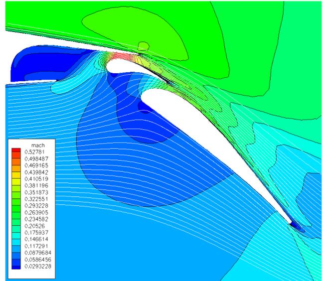
Fig.9: CFD (2D RANS) simulation of flow around a fixed vane flap section
