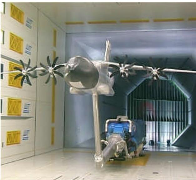
Fig.8: Powered A400M High-Lift complete model in the DNW-LLF windtunnel
