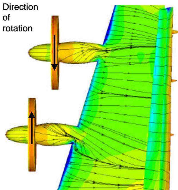
Fig. 4: Effect of propeller wake on wing pressure distribution and streamlines (3D RANS CFD)
