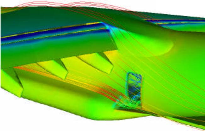
Fig. 10: CFD (3D RANS) assessment of the downstream flow quality behind the complete aircraft in high-lift configuration [1]
