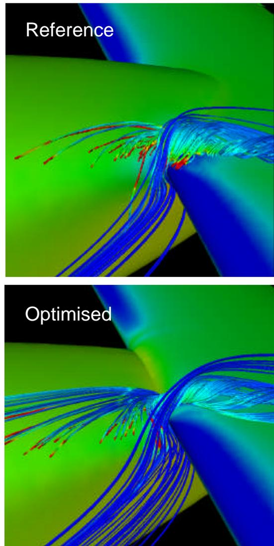
Fig 3: 3D-Flow topology at the leading-edge/nacelle intersection (3D RANS CFD at high A/C incidence)
