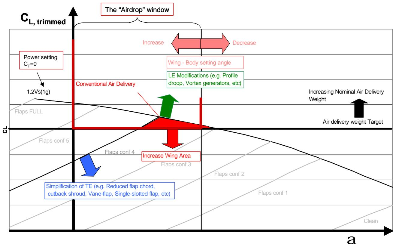
Fig.2: “The Airdrop Diagram” – Design target for the high-lift performance
