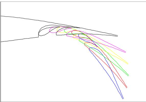
Fig.6: Fixed Vane Flap on Dropped Hinge Kinematics deployment path principle
