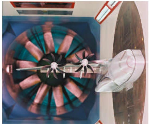
Fig.7: Powered A400M High-Lift halfmodel in the Airbus Low-Speed Windtunnel Bremen
