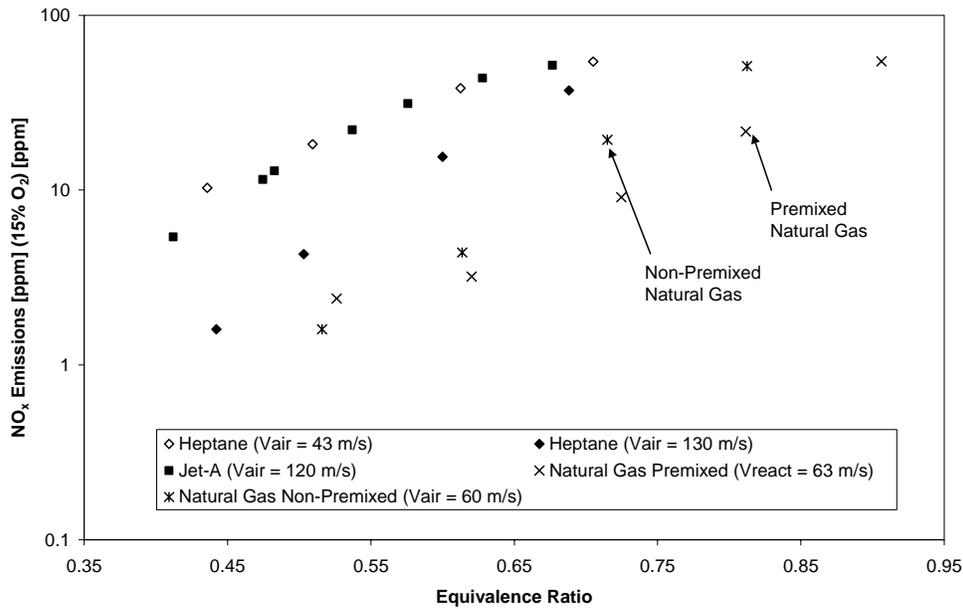
Figure 5. Corrected  $\text{NO}_x$  emissions ( $15\% \text{O}_2$ ) obtained with straight-walled fuel injector with Jet-A and heptane fuels for various discharge air velocities. Emissions with natural gas are shown for comparison.
