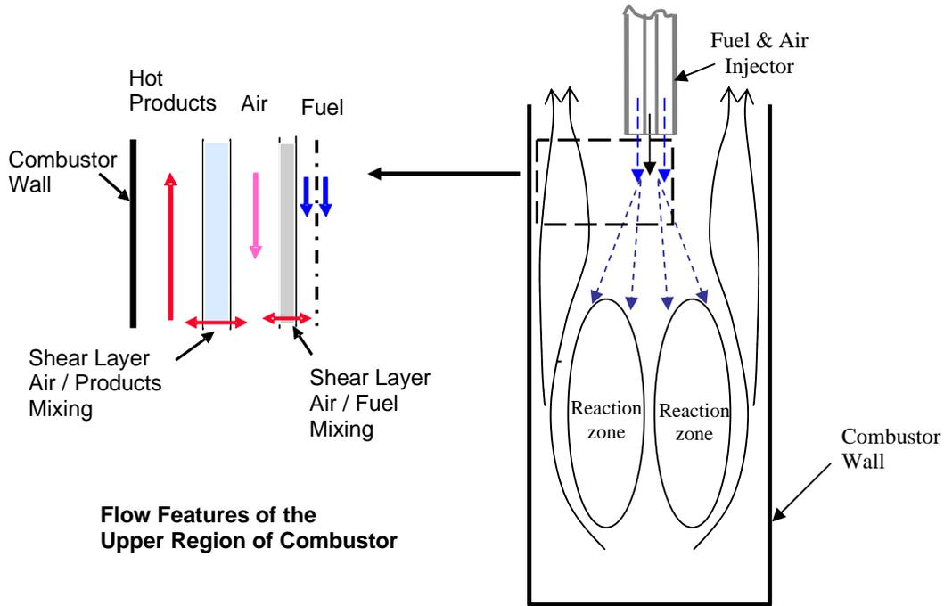
Figure 1. A schematic of SPRF (right) with the flow features of the upper region of the combustor (left).
