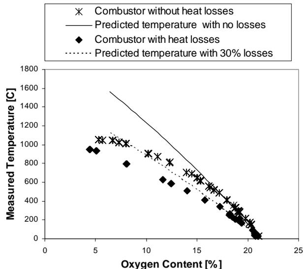
Figure 10: Measured temperature for varying distance from the combustor exit plane as a function of oxygen content
