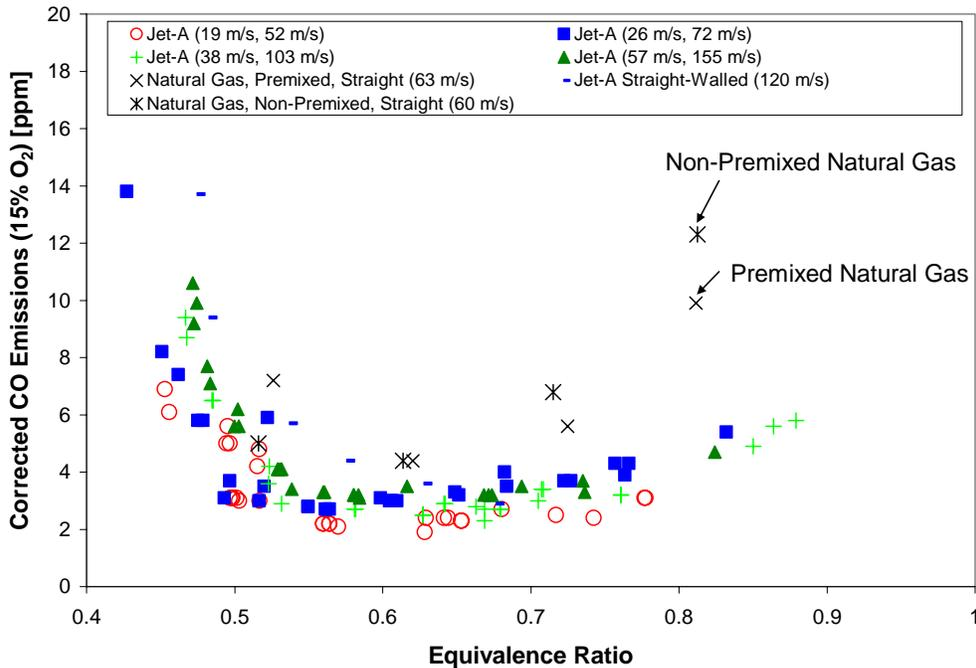
Figure 9. Corrected CO emissions (15% O<sub>2</sub>) for the venturi injector with Jet-A fuel over various air flow rates. The velocity indications are as in Fig. 8.
