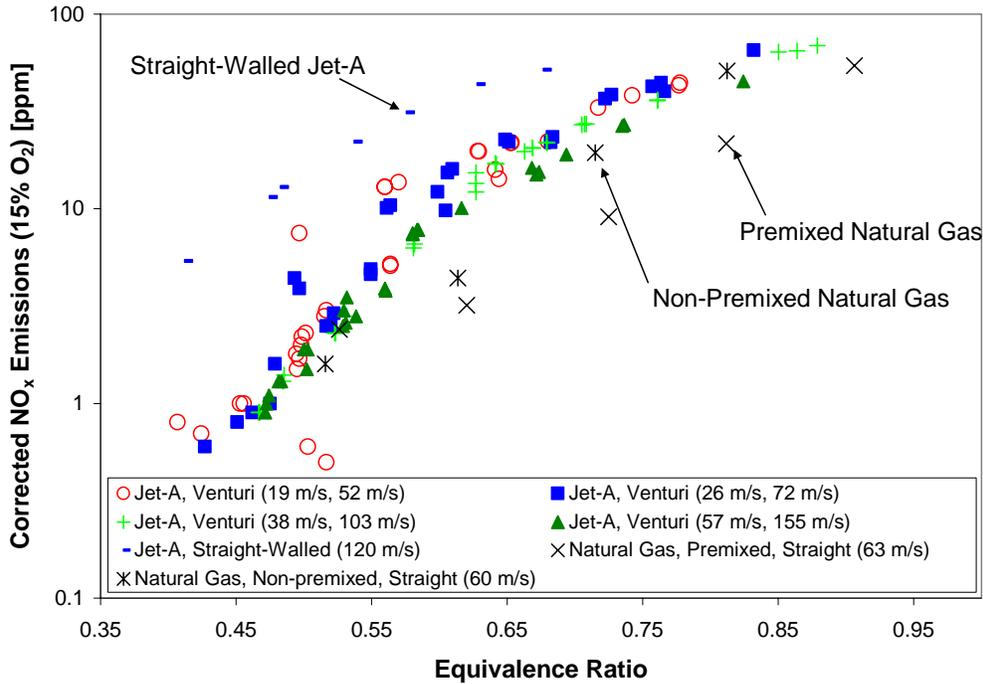
Figure 8. Corrected NO<sub>x</sub> emissions (15% O<sub>2</sub>) for the venturi injector with Jet-A fuel over various air flow rates. Both discharge and throat velocities in the venturi injector are indicated. Results obtained with the straight-walled injector operating with natural gas were included for comparison. In the non-premixed mode the velocity is that of the injected air whereas in the premixed mode the velocity is that of the reactants (both air and fuel).
