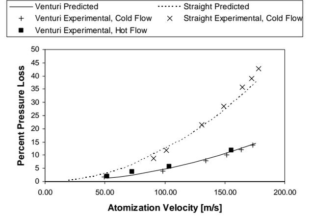
Figure 7. Predicted and measured pressure loss across the injector as a function of velocity at the atomization zone for the straight-walled and venturi injectors.
