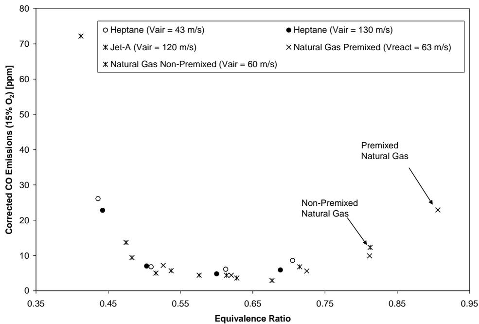
Figure 6. Corrected CO emissions ( $15\% \text{O}_2$ ) obtained with straight-walled fuel injector and Jet-A and heptane fuels for various air injection velocities. Emissions with natural gas operation are shown as well for reference.
