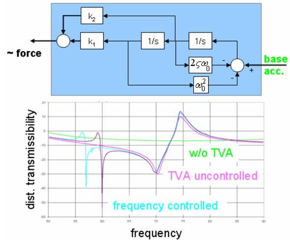
**Fig. 5** Robust disturbance rejection control
