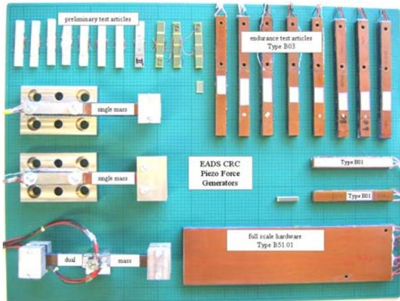
**Fig. 3** Piezo-TVA prototype line
