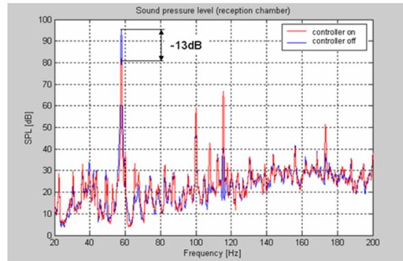
**Fig. 9** Noise reduction of 1BPF-TVA at 58Hz
