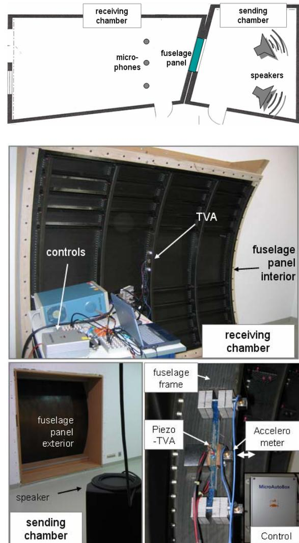
**Fig. 6** Transmission loss test suite
