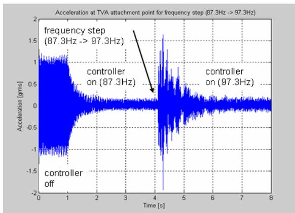
**Fig. 8** Transient behaviour due to step change in excitation frequency
