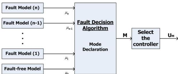
Fig. 3. Fault tolerant control strategy using mode switching
