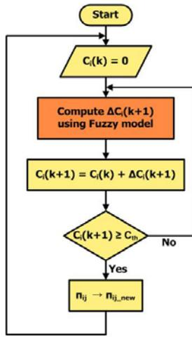
Fig. 2. The flowchart of fuzzy-tuning algorithm
