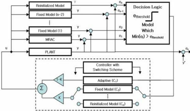
Fig. 6. Controller structure of MMAC
