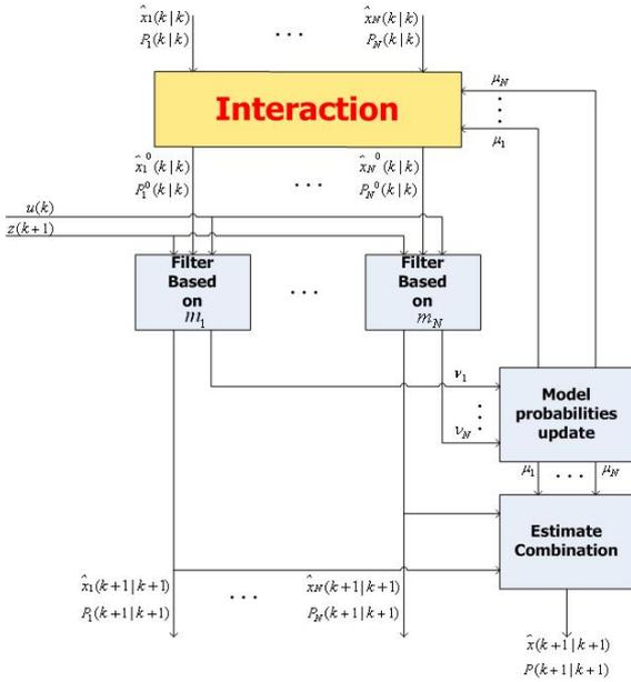
Fig. 1. Structure of the IMM filter
