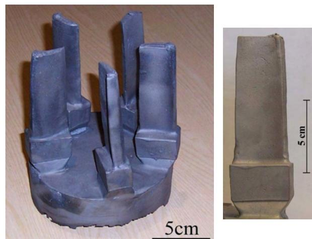
Fig. 4. Investment cast Nb-base silicide blade cluster (left) and blade (right).
