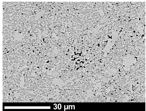
Fig. 7. SEM micrograph (BSE mode) of the MA processed and HIP'ed MoNbSiB alloy with Mo(ss) (bright), intermetallics (grey) and undesired silica (black).
