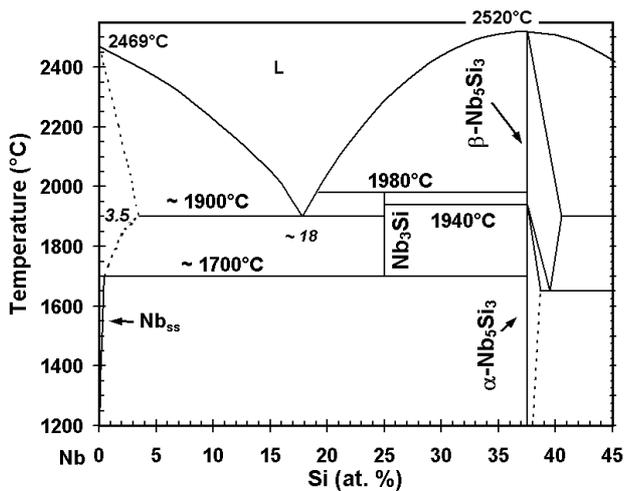
Fig. 2. Nb-rich part of the binary Nb-Si phase diagram (after [13]).
