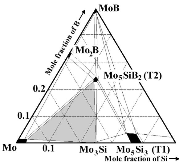
Fig. 1. Mo-rich part of the isotherm section at 1600°C of the Mo-Si-B phase diagram (after [8]). The shaded area is the Mo-T2-Mo<sub>3</sub>Si three phase region.
