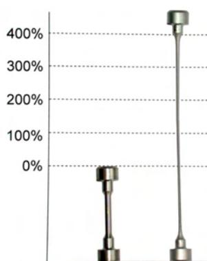
Fig. 8. Comparison of undeformed (left) and deformed (right; 1400°C and  $10^{-4} \text{ s}^{-1}$ ) HIP'ed MoNbSiB tensile sample.
