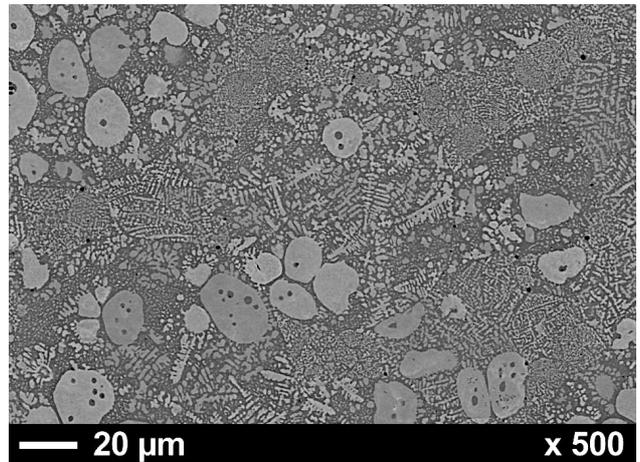
Fig. 6. SEM micrograph in backscattered electrons imaging mode (BSE) of the gas-atomised and HIP'ed Mo-Si-B alloy with Mo(ss) (bright), intermetallics (grey) and silica (dark).
