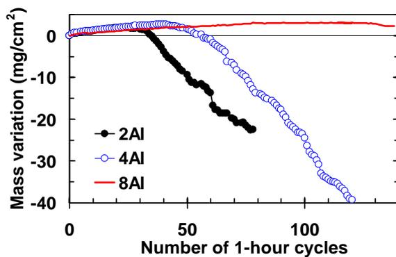
Fig. 12. Cyclic oxidation (1 h cycles) at 815°C of Nb-base silicide alloys of same composition, except for the Al content (given in at. %).
