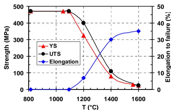
Fig. 9. Dependence of yield strength (YS), UTS, and fracture elongation on temperature of the HIPed Mo-Si-B alloy.
