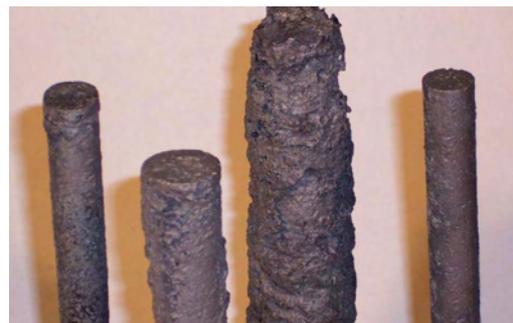
Fig. 3. Investment cast Nb-base silicide bars (diameter: 10 to 30 mm) showing the chemical interaction between mould and melt.
