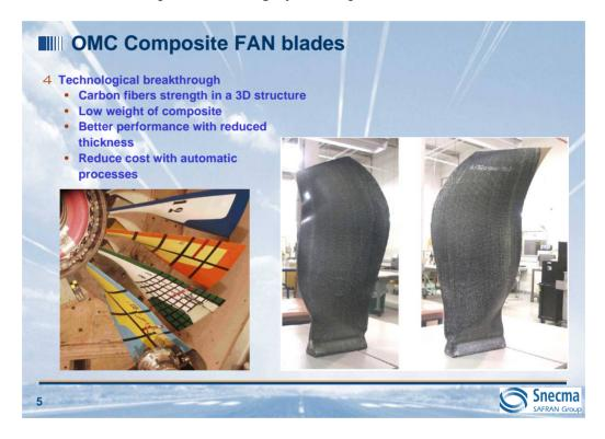
This three-dimension weaving technique is used to create a web of carbon fibers with evolving thickness which is then placed in a mould to inject resin (RTM process). The part thus obtained has the advantages of the carbon fiber resistance in three-dimension, the lightness of the composite and the possibility of complex shapes. In this technology, the two main operations, weaving and injection of resin are automated, which makes it a cheaper technology than the ones it will replace.
