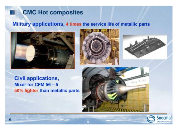
This type of material has already demonstrated its remarkable endurance life for military applications (more than 4 times the life of metallic parts), and particularly its excellent resistance to heat and oxidation. This resistance is due to the self-cicatrizing design of the material, which makes it original.
