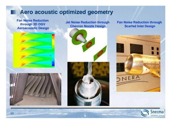
Above this, the decrease in noises at source depends on the optimization of geometry in order to prevent turbulence and interactions. On the FAN side, this leads to very complex "large chord swept blade" geometries, associated to optimized OGV geometries in order to limit wake interactions.
