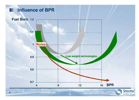
To improve the engine efficiency, the best solution is to increase the dilution ratio to the optimum, when the gain in propulsion efficiency is compensated by the increase in the engine diameter and the resulting weight and drag increase. The use of lighter technologies will move this optimum upwards. With today's technologies, the optimum dilution ratio is approximately 8, it will be  $\approx$  10-12 around 2012. It is difficult to forecast dilution ratios for 2017.
