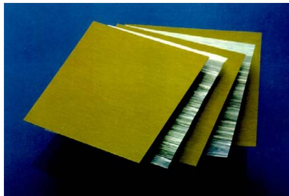
Figure 1: Typical GLARE® lay-up
