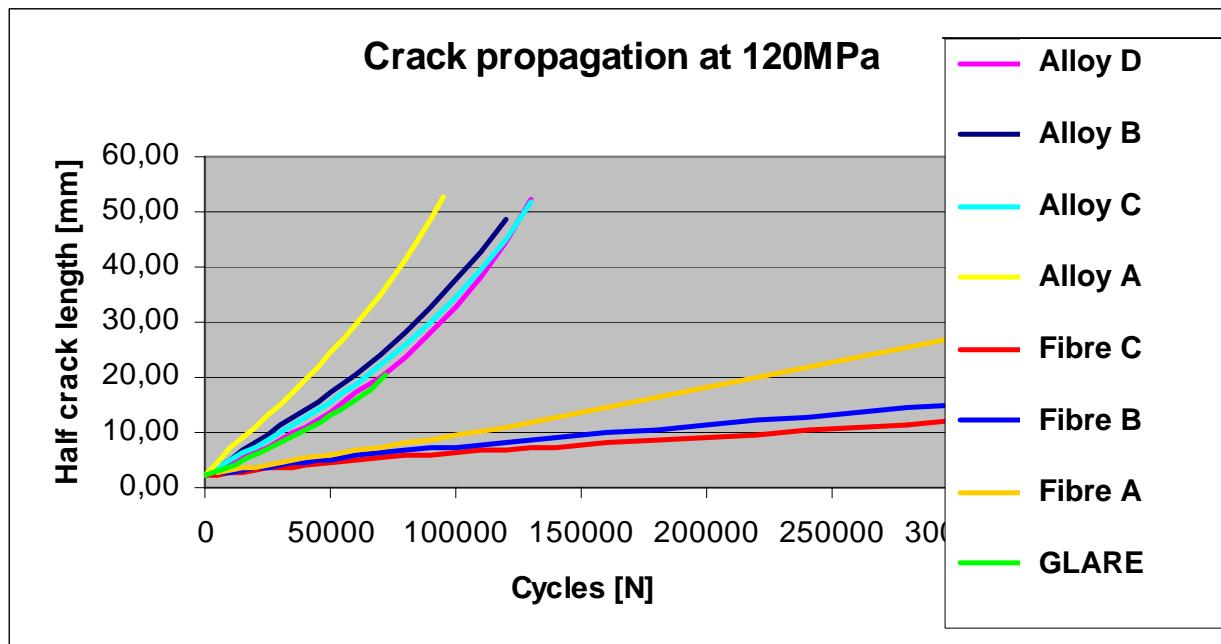
Figure 8: Crack propagation behaviour of new laminates
