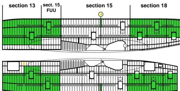
Figure 2: GLARE® (green) application at Airbus A380 [11]
