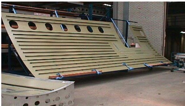
Figure 7: GLARE® fuselage panel
