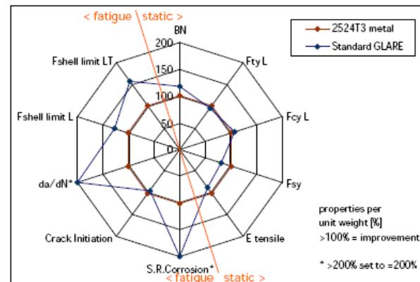
Figure 3: Improved properties of GLARE® in comparison to 2524 T3
