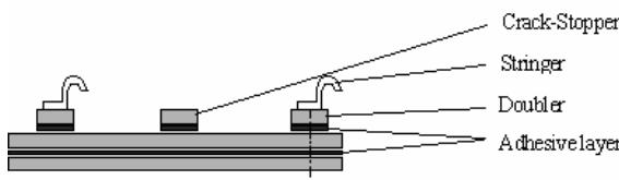
Figure 4: Design principle of Metal Laminates
