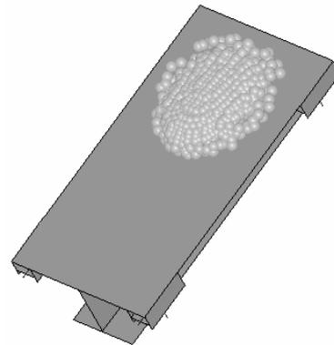
Figure 2. Numerical model of the test carried out for bird characterisation.
