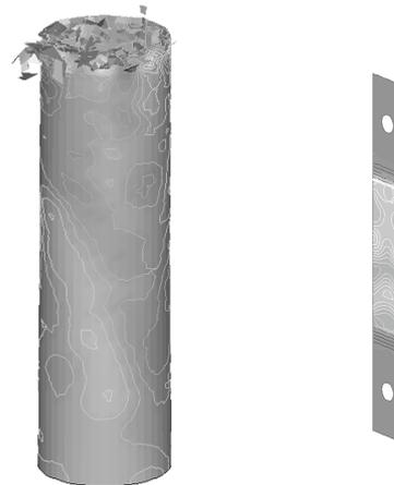
Figure 3. Vertical crush test (LHS) and dynamic tensile test (RHS).
