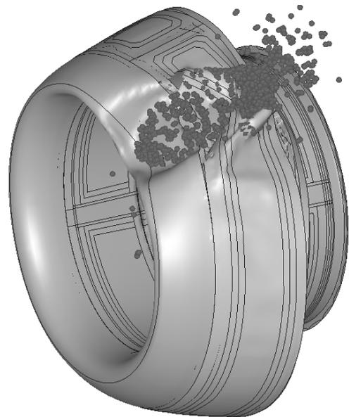
Figure 4. Birdstrike onto a turbofan-engine intake.
