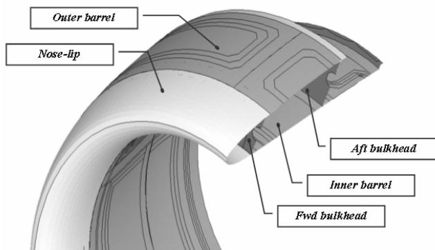
Figure 1. Turbofan intake structural scheme.
