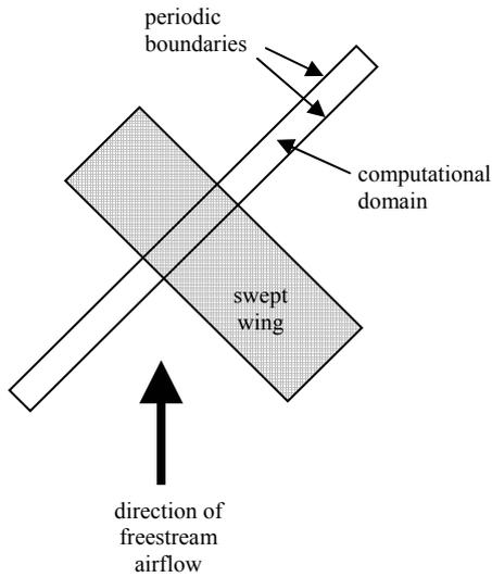
Fig. 2. Top view of swept wing and computational domain (not to scale).
