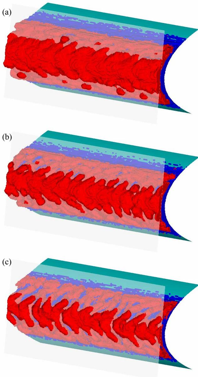
Fig. 5. Predicted lobster tail (scallop) ice shapes forming on a swept wing with a freezing range parameter of 3.0 and varying sweep angle.
