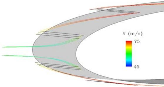
Fig. 3. Predicted streamlines coloured according to the flow velocity for a sweep angle of  $45^\circ$ .
