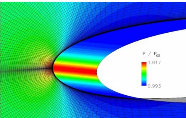
Fig. 4. Predicted flow field for a sweep angle of  $45^\circ$ . The computational grid used for the simulation is also shown. (a) velocity contours at the periodic boundary (b) pressure contours at the periodic boundary and wing surface
