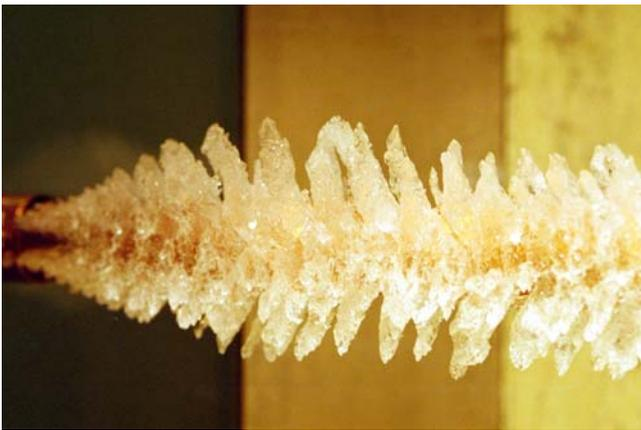
Fig. 1. Experimental lobster tail ice shape (courtesy of M. Oleskiw of NRC, Canada).
