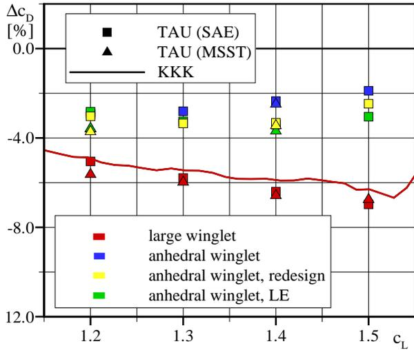
**Fig. 20** Drag Reduction Of Different Wing Tip Devices Relative To Küchemann,  $M = 0.2$ ,  $Re = 7.2 \cdot 10^6$
