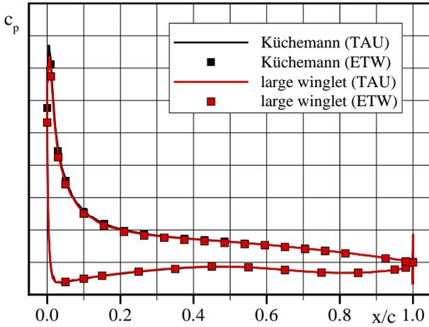
**Fig. 5** Pressure Distributions On Spanwise Station  $\eta = 0.47$ ,  $c_L = 1.0$ ,  $M = 0.2$ ,  $Re = 7.2 \cdot 10^6$
