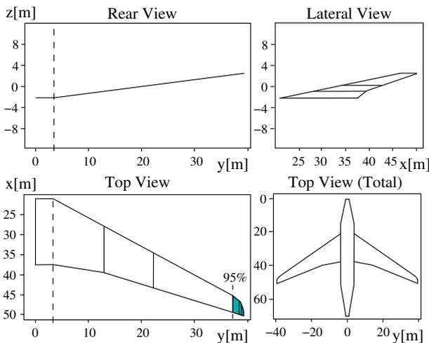
**Fig. 1** Schematic of wing planform with reference wing tip
