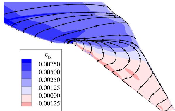
Fig. 10 Streamtraces and  $c_{fx}$  contour plot for anhedral winglet,  $c_L = 0.9$ ,  $M = 0.2$ ,  $Re = 7.2 \cdot 10^6$
