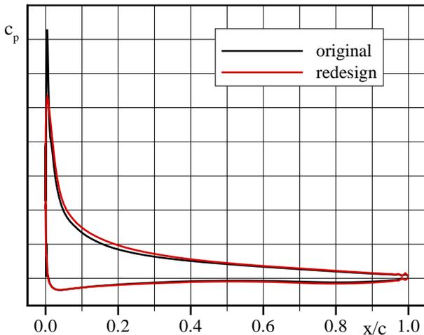
**Fig. 12** Pressure distributions of large winglet using original and redesigned airfoils,  $\eta = 1.04$ ,  $\alpha = 12.5^\circ$ ,  $M = 0.2$ ,  $Re = 7.2 \cdot 10^6$
