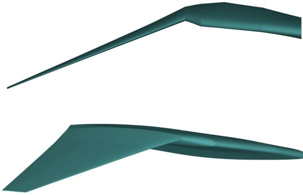
**Fig. 2** Visualisation Of The Anhedral Winglet From Front View (**Top**) And Lateral View (**Bottom**)
