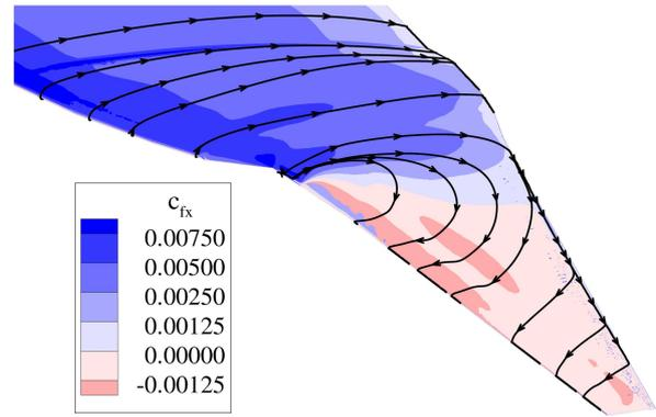
**Fig. 16** Streamtraces and  $c_{fx}$  contour plot for anhedral winglet with redesigned airfoils,  $c_L = 1.0$ ,  $M = 0.2$ ,  $Re = 7.2 \cdot 10^6$
