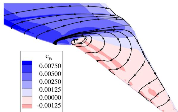
Fig. 11 Streamtraces and  $c_{fx}$  contour plot for anhedral winglet,  $c_L = 1.0$ ,  $M = 0.2$ ,  $Re = 7.2 \cdot 10^6$
