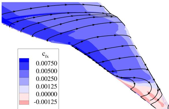
**Fig. 15** Streamtraces and  $c_{fx}$  contour plot for anhedral winglet with redesigned airfoils,  $c_L = 0.9$ ,  $M = 0.2$ ,  $Re = 7.2 \cdot 10^6$
