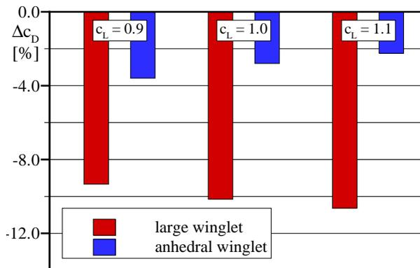
Fig. 9 Drag Reduction Of Different Wing Tip Devices Relative To Küchemann, TAU results,  $M = 0.2$ ,  $Re = 7.2 \cdot 10^6$
