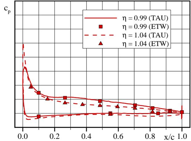
**Fig. 7** Pressure Distribution Of Large Winglet,  $c_L = 1.0$ ,  $M = 0.2$ ,  $Re = 7.2 \cdot 10^6$
