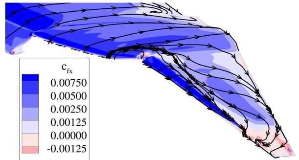
**Fig. 23** Streamtraces and  $c_{fx}$  contour plot for anhedral winglet with leading edge device, MSST,  $c_L = 1.4$ ,  $M = 0.2$ ,  $Re = 7.2 \cdot 10^6$
