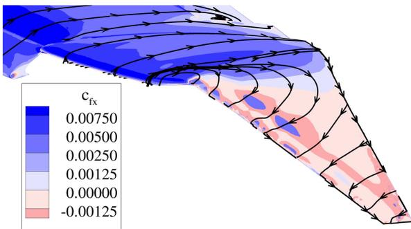
**Fig. 21** Streamtraces and  $c_{fx}$  contour plot for anhedral winglet, MSST,  $c_L = 1.4$ ,  $M = 0.2$ ,  $Re = 7.2 \cdot 10^6$
