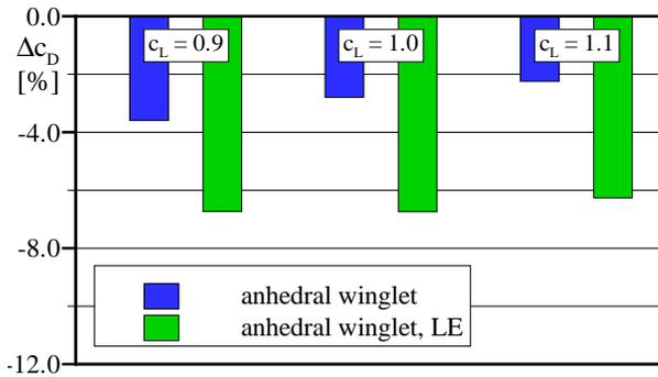
**Fig. 17** Drag Reduction Of Different Wing Tip Devices Relative To Küchemann, TAU results,  $M = 0.2$ ,  $Re = 7.2 \cdot 10^6$
