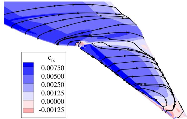
**Fig. 19** Streamtraces and  $c_{fx}$  contour plot for anhedral winglet with leading edge device,  $c_L = 1.0$ ,  $M = 0.2$ ,  $Re = 7.2 \cdot 10^6$
