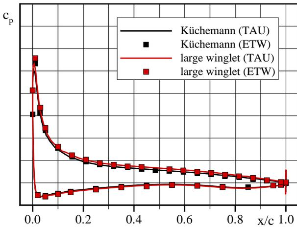
**Fig. 6** Pressure Distributions On Spanwise Station  $\eta = 0.95$ ,  $c_L = 1.0$ ,  $M = 0.2$ ,  $Re = 7.2 \cdot 10^6$
