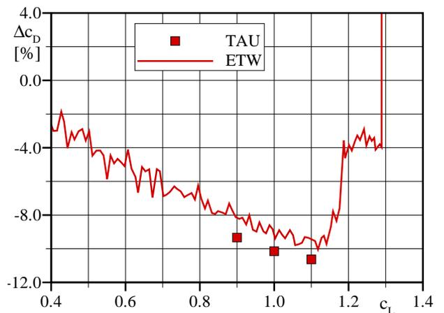
**Fig. 8** Drag Reduction Of Large Winglet Relative To Küchemann,  $M = 0.2$ ,  $Re = 7.2 \cdot 10^6$
