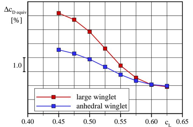
**Fig. 4** Equivalent Drag Reduction Relative To Küchemann, TAU result,  $M = 0.85$ ,  $Re = 54.2 \cdot 10^6$
