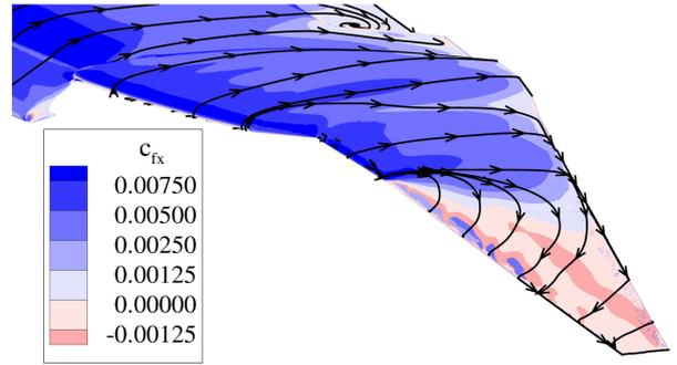
**Fig. 22** Streamtraces and  $c_{fx}$  contour plot for anhedral winglet with redesigned airfoils, MSST,  $c_L = 1.4$ ,  $M = 0.2$ ,  $Re = 7.2 \cdot 10^6$
