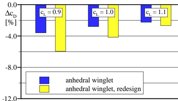
**Fig. 14** Drag Reduction Of Different Wing Tip Devices Relative To Küchemann, TAU results,  $M = 0.2$ ,  $Re = 7.2 \cdot 10^6$
