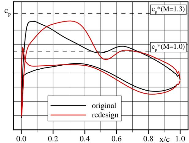
**Fig. 13** Pressure distributions of large winglet using original and redesigned airfoils,  $\eta = 1.04$ ,  $c_L = 0.5$ ,  $M = 0.85$ ,  $Re = 54.2 \cdot 10^6$
