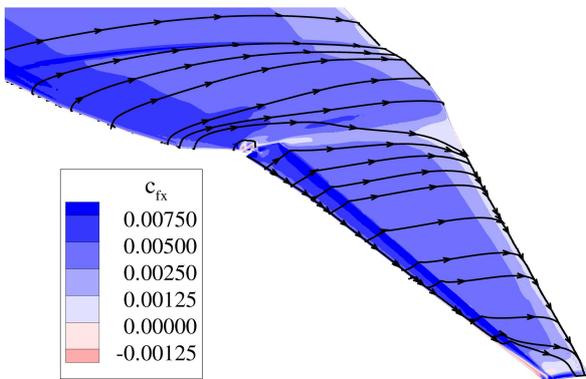
**Fig. 18** Streamtraces and  $c_{fx}$  contour plot for anhedral winglet with leading edge device,  $c_L = 0.9$ ,  $M = 0.2$ ,  $Re = 7.2 \cdot 10^6$
