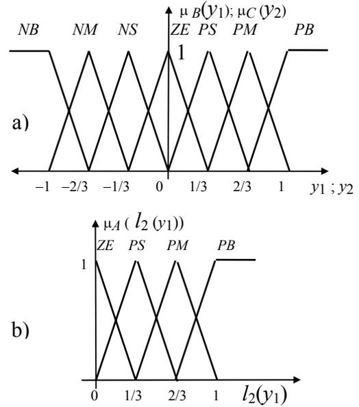
Fig. 2. Triangular membership functions for: a) scaled input variables  $y_1, y_2$  and b)  $l_2(y_1)$ .
