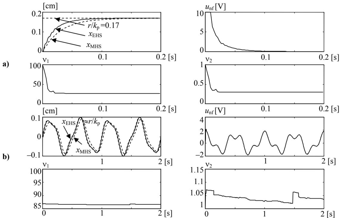
Fig. 5. Neuro-fuzzy controlled EHS,  $F_f \neq 0$ , comparison with MHS. Desired ( $r/k_p$ ) and actual ( $x$ ) piston displacements. a) step reference; b) sinusoidal combination reference.
