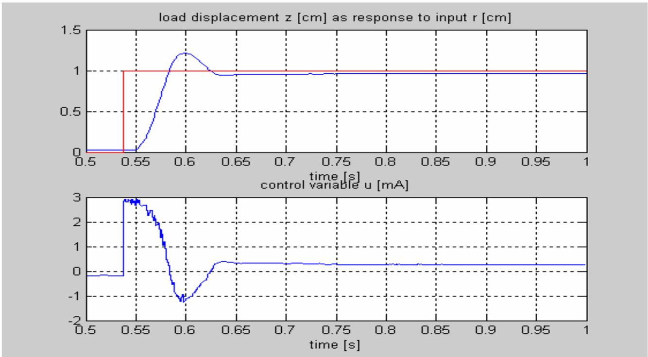
Fig. 7. Experimental tests, FSNC algorithm. Overshoot 21%, time constant 0.03 s, stationary error 4%.
