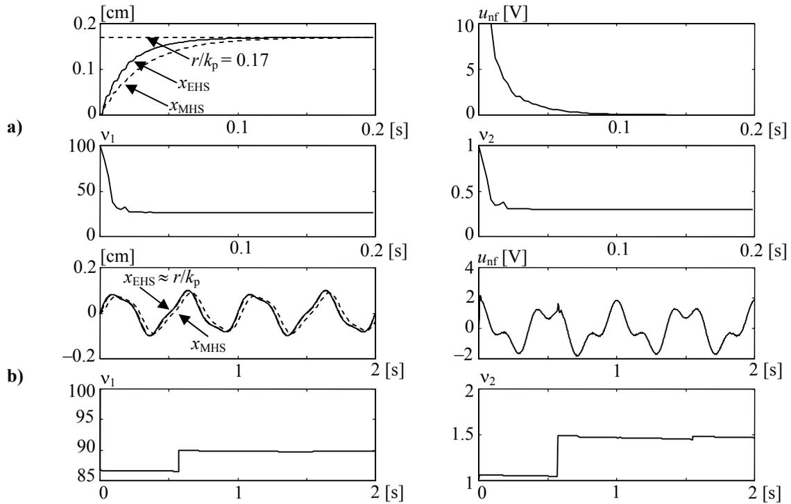
Fig. 4. Neuro-fuzzy controlled EHS,  $F_f = 0$ , comparison with MHS. Desired ( $r/k_p$ ) and actual ( $x$ ) piston displacements. a) step reference; b) sinusoidal combination reference.
