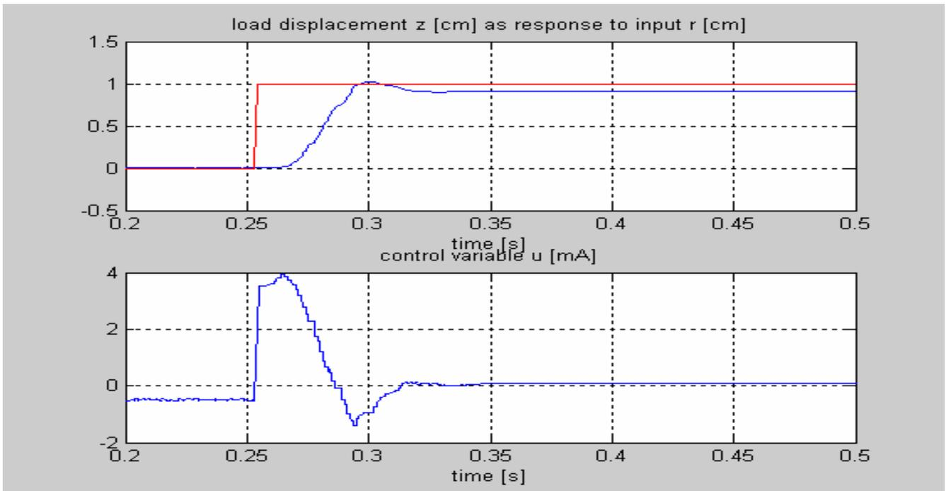
Fig. 6. Experimental tests, LQR algorithm. Overshoot 1.5 %, time constant 0.032 s, stationary error 10 %.
