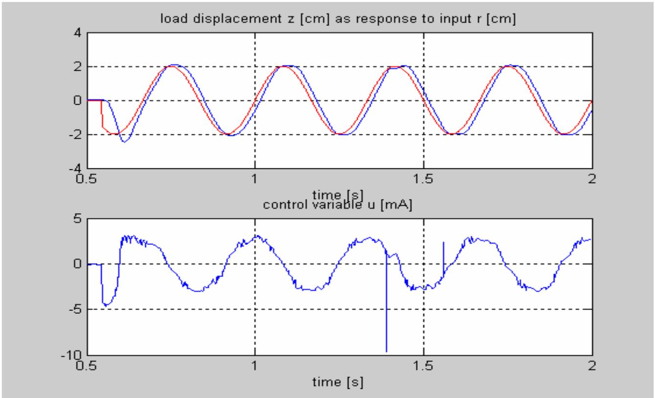
Fig. 9. Experimental tests, FSNC algorithm: sinusoidal reference response (amplitude 2 cm, frequency 3 Hz). Time delay 0.016 s, 0% attenuation.
