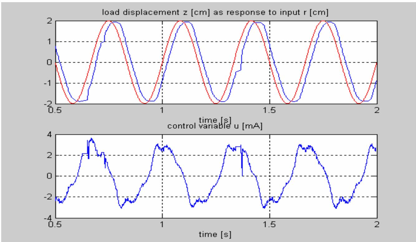
Fig. 8. Experimental tests, LQG algorithm: sinusoidal reference (amplitude 2 cm, frequency 3 Hz). Time delay 0.025 s, 10 % attenuation.
