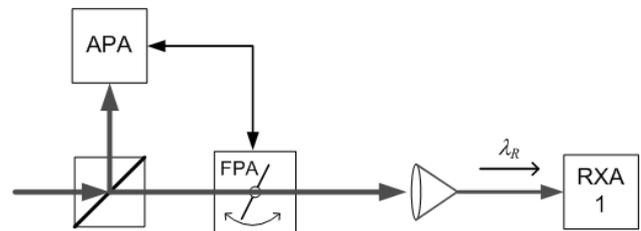
**Fig. 7 Beaconless receiver concept: The Rx-coms.-signal is split. One part is used on the tracking receiver (APA) to detect the beam alignment and to control the fine pointing assembly (FPA). The other part is focused on the data receive assembly (RXA).**
