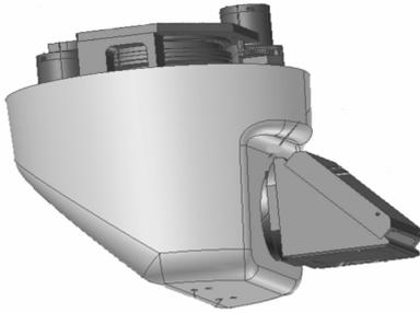
**Fig. 9 DLR-design of an optical terminal antenna with CPA. This system was proven for a 1250 Mbps downlink from a slowly moving stratospheric balloon-platform, but can be adapted for avionic applications. The pointing accuracy of this system is about 0.2 mrad.**
