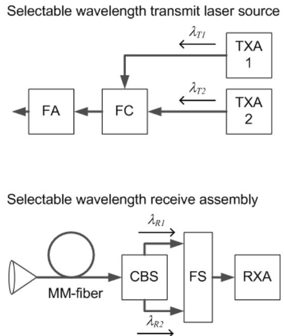
**Fig. 6 Full-duplex system approach with arbitrary connectivity using selectable transmit and receive wavelengths paths (FA: fiber-amplifier, FC: fiber-combiner, TXA: transmit assembly, CBS: chromatic beam splitter, FS: fiber-switch, RXA: receive assembly)**
