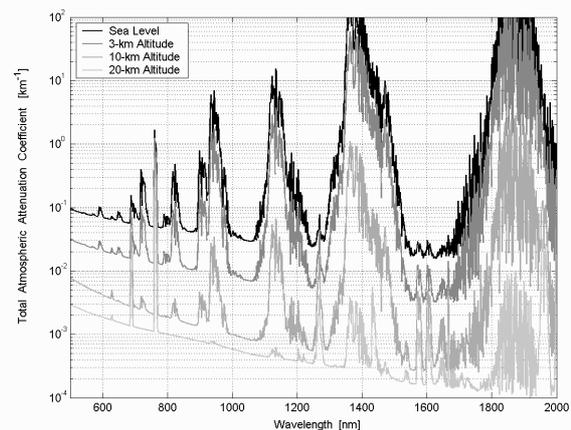
**Fig. 3** Altitude dependant coefficient of clear-sky atmospheric attenuation vs. optical and near-infrared wavelengths. Four different altitudes are considered: sea level (uppermost curve), 3 km, 10 km, 20 km (lowest curve) Attenuation values are averaged over 1 nm [9]
