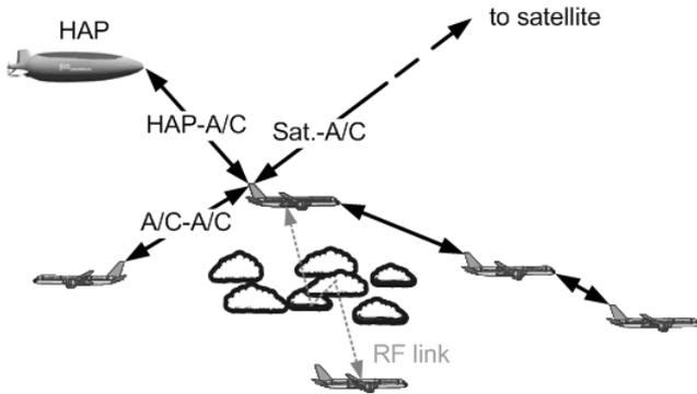
**Fig. 1 Application scenarios for aeronautical optical links**
