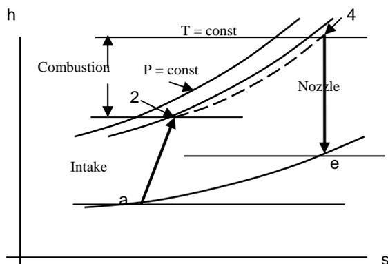
**Fig.4.** Introduction of losses in the ideal cycle, the “Semi-ideal”scramjet in an enthalpy (h) – entropy (s) diagram
