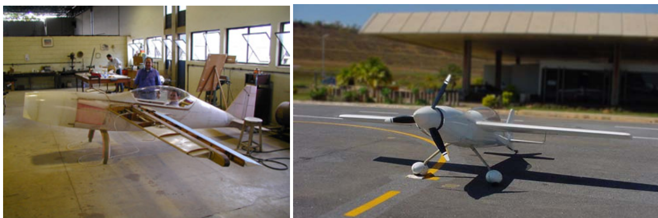
Figure 2 – Prototype of the aircraft CEA-308 in construction and in operation
