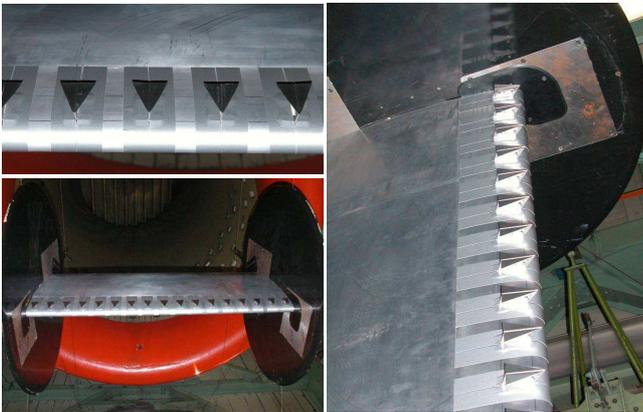
**Fig. 11** Experimental setup of the 2.5 dimensional validation tests of the active vortex generator array.
