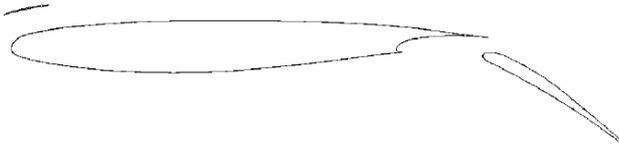
**Fig. 7** Profile Geometry, AVG wing landing configuration.
