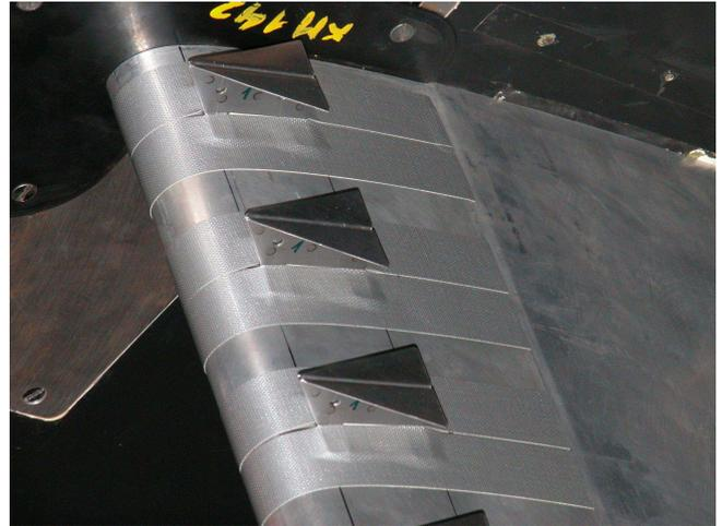
**Fig. 2** Picture of the experimental setup at VZLU, showing the vortex generator array at the leading edge of the wing profile.
