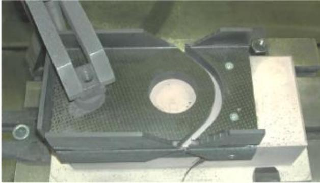
Fig. 10. Machining of the lug shape.
