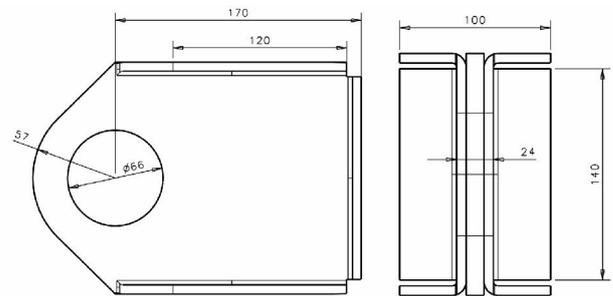
Fig. 1. Lug geometry and main dimensions
