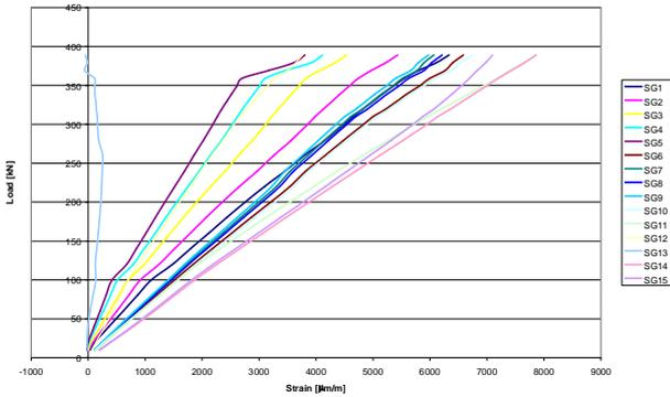
Fig. 18. Load-strain response of the second specimen.
