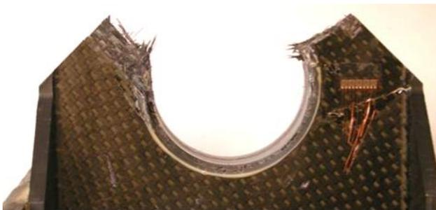
Fig.20. Failure of the second lug specimen
