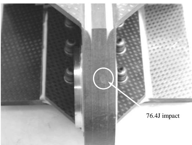
Fig. 24. Impact damage of the fifth specimen.
