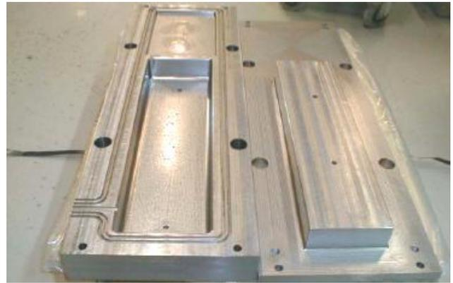
Fig. 8. Tooling for the lug parts.
