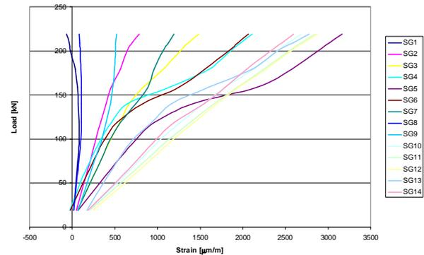
Fig. 15. Load-strain response of the first lug specimen.
