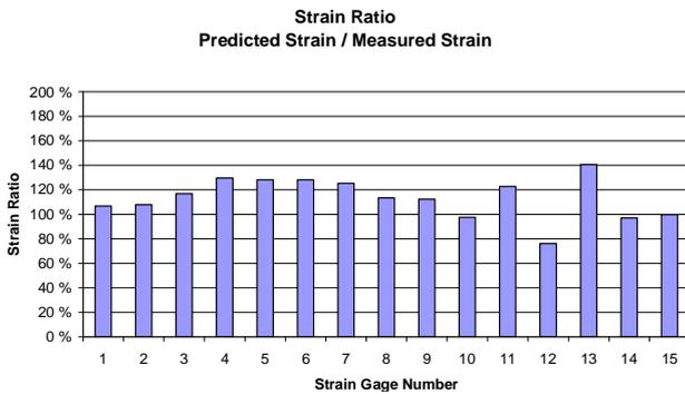
Fig. 19. Strain ratio of the second specimen.
