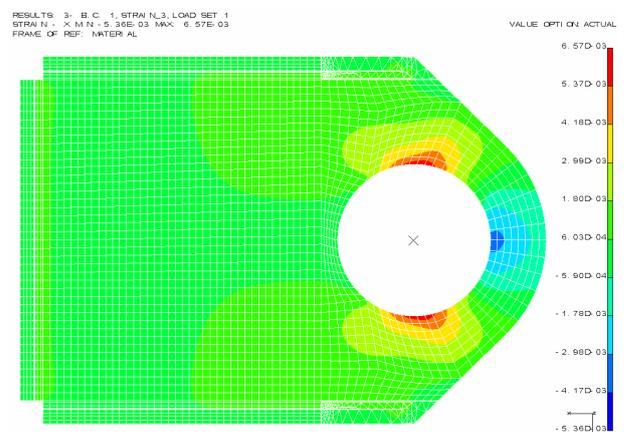
Fig. 5. Normal longitudinal strains in the lug.
