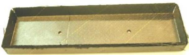
Fig. 7. Preform for the outer lug parts.
