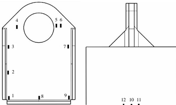
Fig. 13. Strain gauges for the lug 1 specimen.
