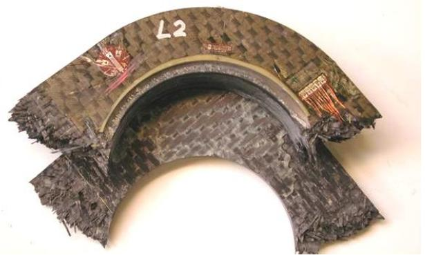
Fig. 21. Debonded parts of the second lug specimen.
