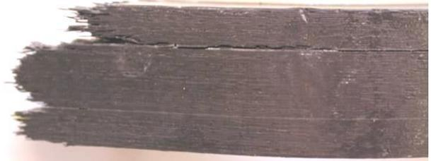
Fig. 26. Partially debonded parts of the fifth specimen.
