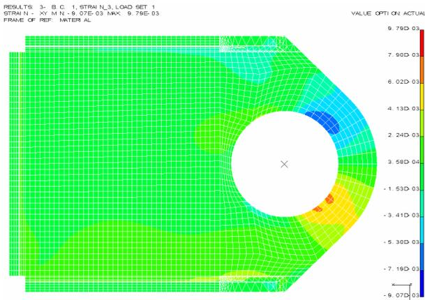
Fig. 6. Shear strains in the lug.
