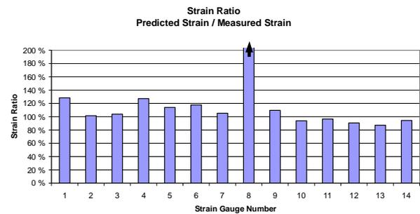
Fig. 16. Strain ratio in the first lug specimen
