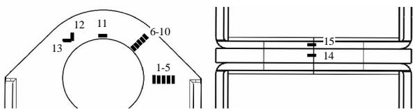
Fig. 14. Strain gauges for the lug 2 specimen.
