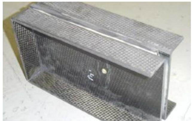
Fig. 9. Bonded lug structure before machining.
