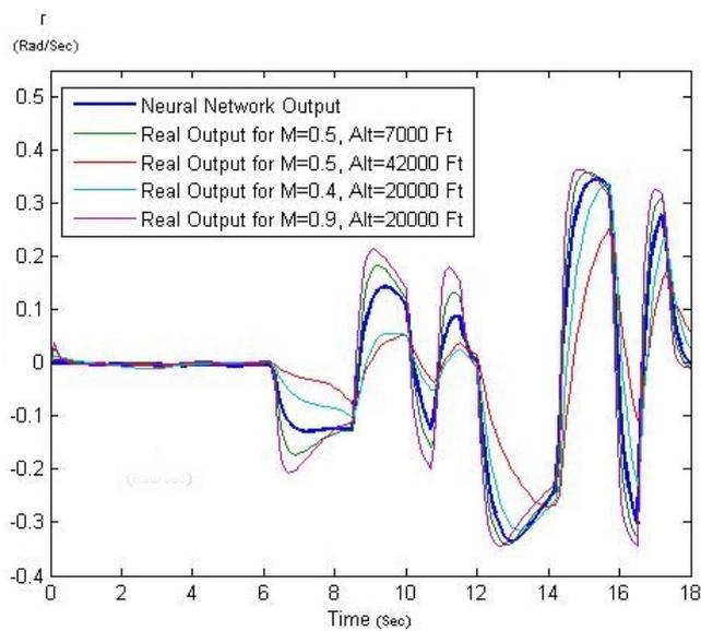
Fig. 6. Mach and Altitude Effect on Yaw Rate Response
