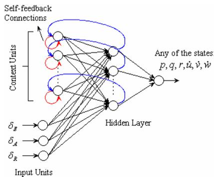
Fig. 1. Modified Elman Network Architecture
