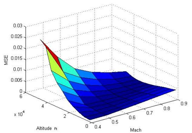
Fig. 7. Mean Squared Error of Yaw Rate Network versus Mach and Altitude
