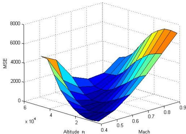
Fig. 8. Mean Squared Error of Lateral Acceleration ( $\dot{v}$ ) Network versus Mach and Altitude
