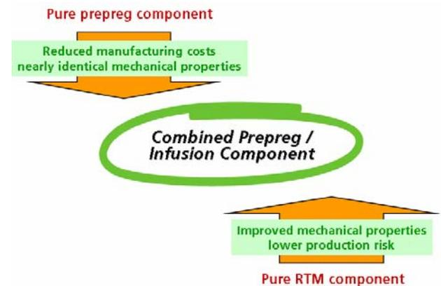
Fig. 1: Comparison of the „Hybrid Fabrication Route“ and the Prepreg and Infusion Technology [5]
