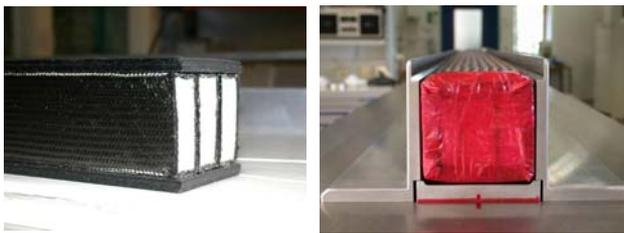
**Fig. 12:** Manufacture of the spar with prepreg belts (left); spar with final wrapping in the tool (right)
