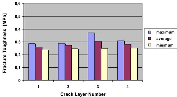
Fig. 7: Distribution of fracture toughness in hybrid-fabricated samples manufactured with a holding time of 90 minutes at 120°C
