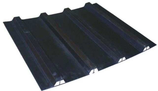
**Fig. 11:** Finished stringer-reinforced prepreg shell made by hybrid fabrication technology
