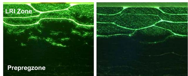
**Fig. 4:** Hybrid sample manufactured at a holding temperature of 120°C (left) and 90°C (right)
