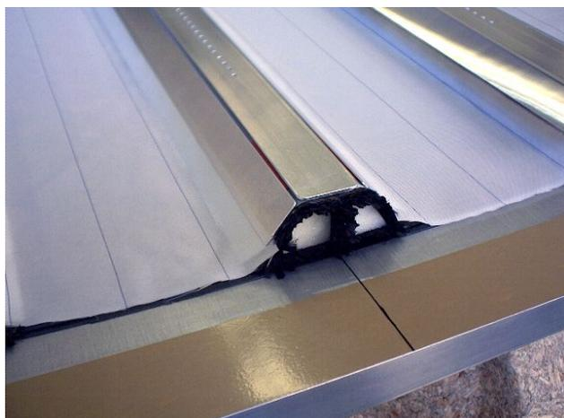
**Fig. 10:** Assembly of the stringers on the prepreg shell with pressure plates
