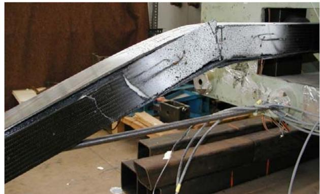
**Fig. 14:** Break point after fracture; top: wet spar with belt detached; bottom: hybrid spar
