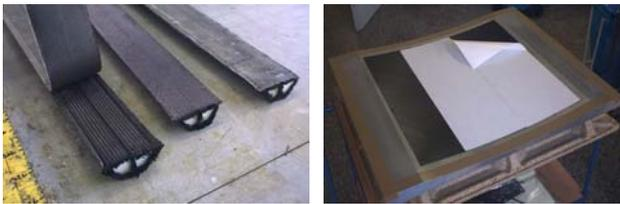
**Fig. 9:** Dry stringer preforms (left) and prepreg shell (right)
