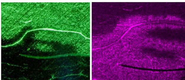
**Fig. 3:** Hybrid sample with green coloured injection resin (left) and purple coloured prepreg resin by EDX (right) [11]
