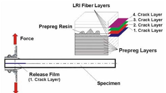
Fig. 6: Description of samples and crack positions
