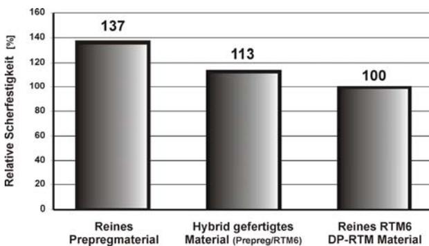
Fig. 4: Standardized interlaminar shear strengths (ILS)
