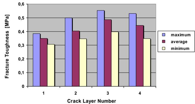
Fig. 8: Distribution of fracture toughness in hybrid-fabricated samples manufactured with a holding time of 30 minutes at 90°C
