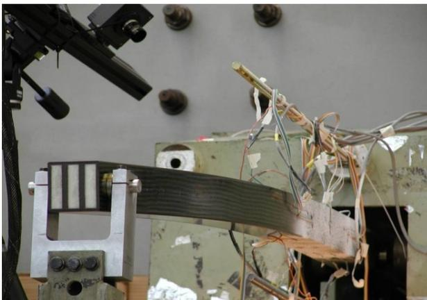
**Fig. 13:** Fracture testing of a spar with prepreg belts
