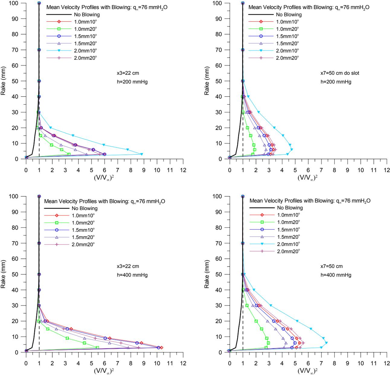
Figure 8 - Analysis All Six Injectors at  $X_3=22 \text{ cm}$  and  $X_7=50 \text{ cm}$  (a)  $h= 200 \text{ mmHg}$  and (b)  $h= 400 \text{ mmHg}$ .
