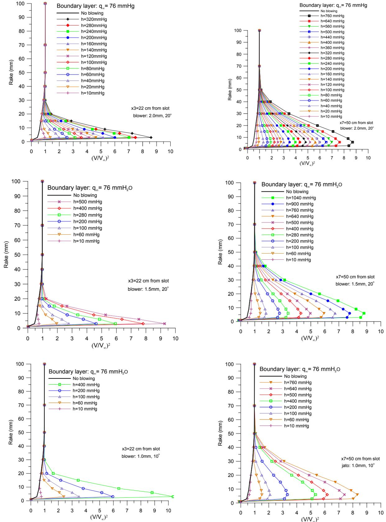
Figure 6- Effect of Blowing on Boundary-layer Profiles on the Test Section Floor at  $X_3 = 22 \text{ cm}$  and  $X_7 = 50 \text{ cm}$  and Several Stagnation pressures : (a) blower:  $2.0 \text{ mm } 20^\circ$ ; (b) blower:  $1.5 \text{ mm } 20^\circ$ ; (c) blower:  $1.0 \text{ mm } 20^\circ$
