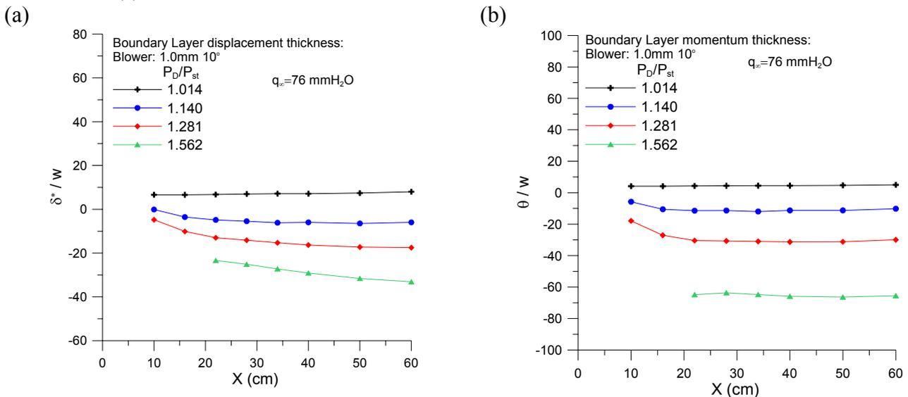
Figure 10 – Boundary-layer Parameters Along the Test Section Floor for Several Blowing Pressure Ratios.  $1.0\text{mm}$  blower set at  $10^\circ$ : (a) Displacement Thickness and (b) Momentum Thickness.
