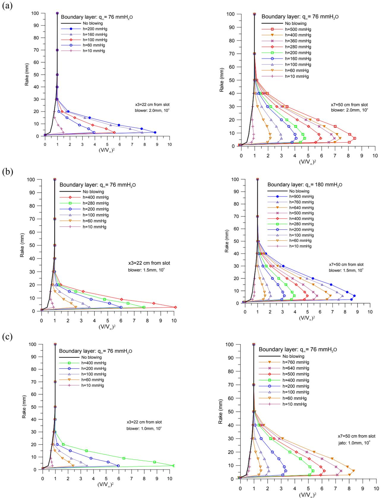
Figure 5 - Effect of Blowing on Boundary-layer Profiles on the Test-section Floor for  $X_3 = 22 \text{ cm}$  and  $X_7 = 50 \text{ cm}$  and several stagnation pressures: (a) blower:  $2.0 \text{ mm } 10^\circ$ ; (b) blower:  $1.5 \text{ mm } 10^\circ$ , (c) blower:  $1.0 \text{ mm } 10^\circ$ .
