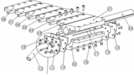
Figure 3: Blower for Boundary-layer Control
