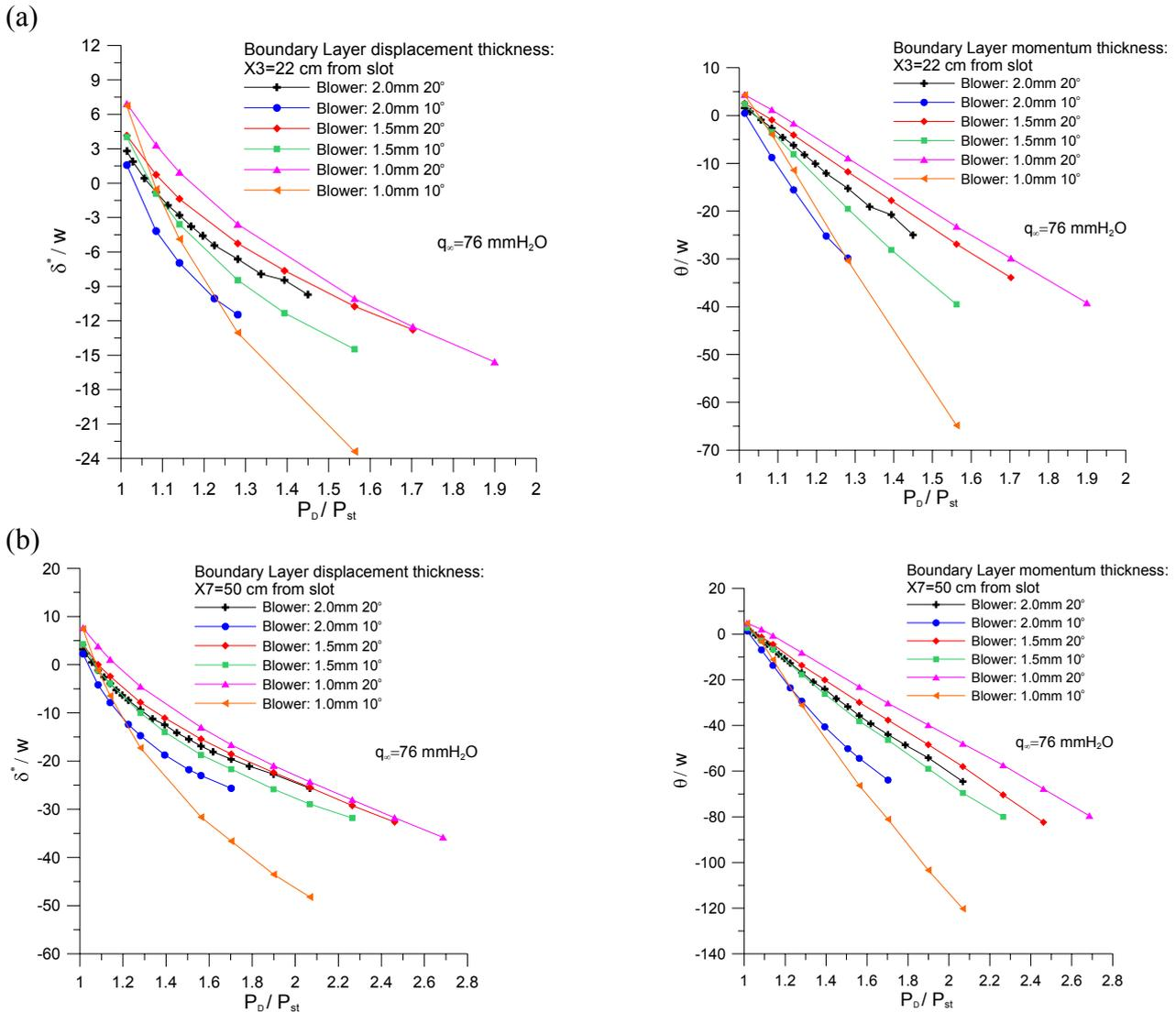
Figure 9: Boundary-layer Displacement,  $\delta^*/w$ , and Momentum Thickness,  $\theta/w$ , for Several Blowing Pressure Ratios at (a)  $X_3=22\text{ cm}$  and (b)  $X_7=50\text{ cm}$ .
