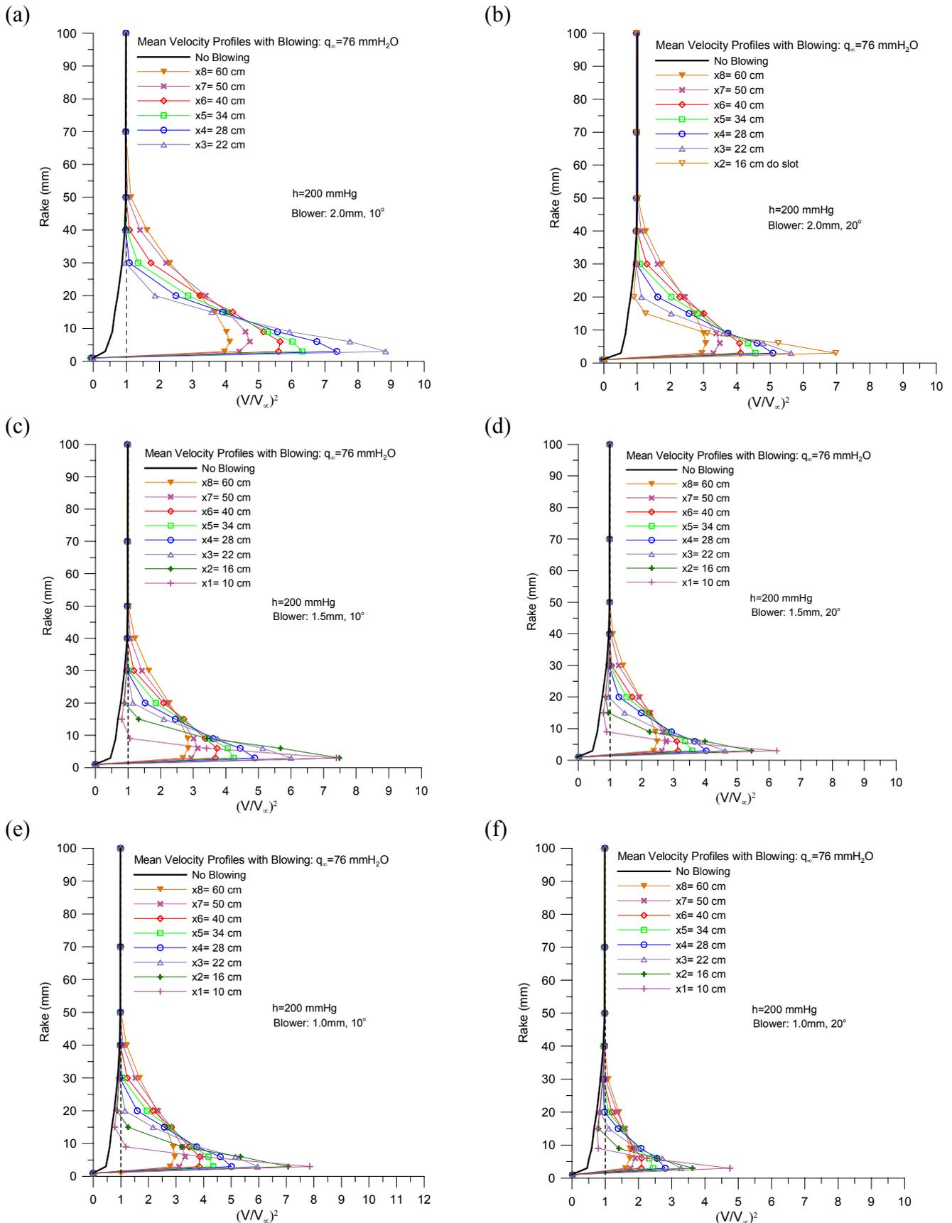
Figure 7- Behavior of Blowing on Boundary-layer Profiles Along the Test Section Floor for  $h = 200 \text{ mmHg}$ : (a)  $2.0 \text{ mm } 10^\circ$ ; (b)  $2.0 \text{ mm } 20^\circ$ ; (c)  $1.5 \text{ mm } 10^\circ$ ; (d)  $1.5 \text{ mm } 20^\circ$ ; (e)  $1.0 \text{ mm } 10^\circ$ ; (f)  $1.0 \text{ mm } 20^\circ$ .
