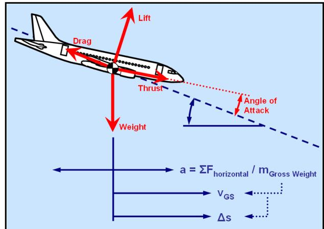
**Fig. 4. Simplified visualization of the flight mechanical model employed.**
