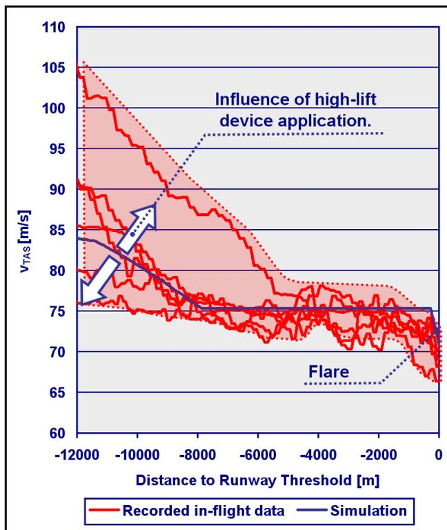
**Fig. 6. True Air Speed validation example (Airbus A320, Airport: LSZH).**
