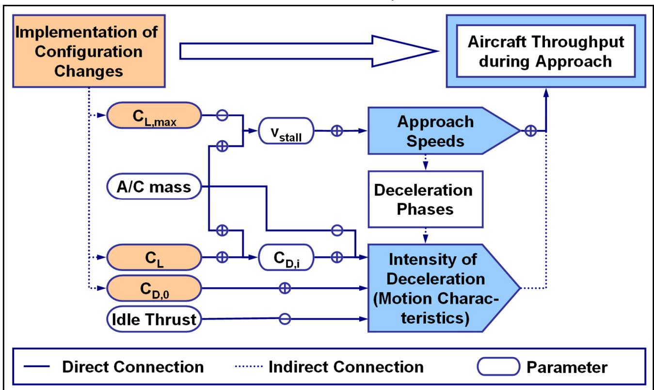
Fig. 7. Direct and indirect correlations between technology or procedure variations and aircraft throughput rates in the approach segment.
