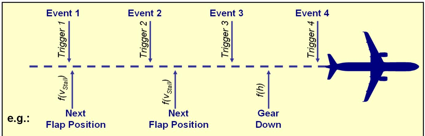
Fig. 5. Generic flight control procedures in the flight guidance simulation.
