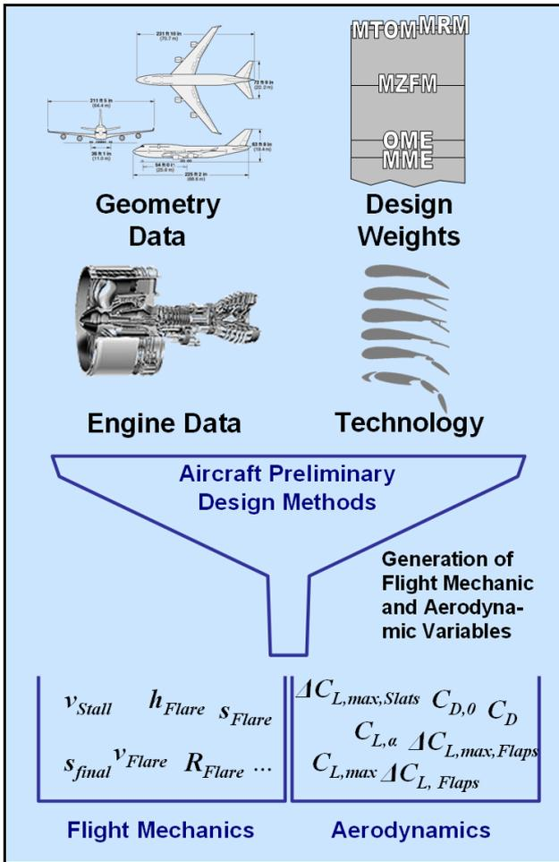
**Fig. 3. Transformation of basic aircraft design parameters into flight mechanics and aerodynamic variables.**
