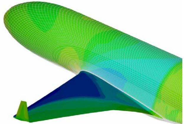
Figure 4: Undeformed CFD model, local  $c_p$  at high  $c_L$  in cruise flight condition
