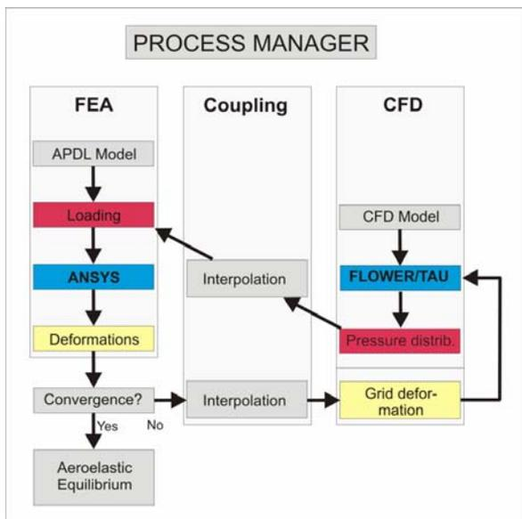
Figure 6: Sequential coupling algorithm
