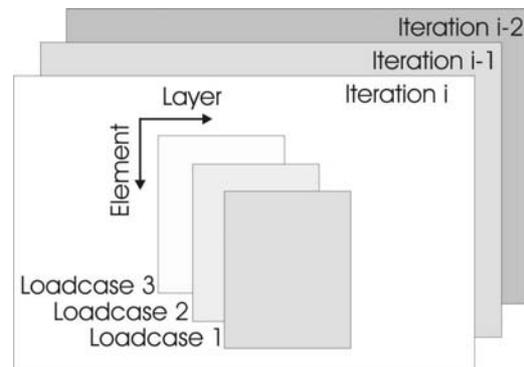
Figure 9: Data Structure of Analysis Results
