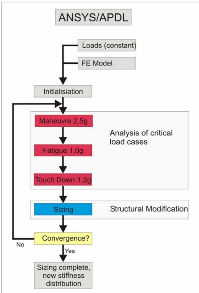
Figure 8: General S\_BOT procedure; presented with the three typical loadcases
