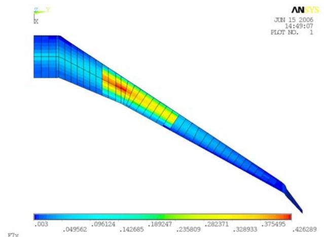
Figure 12: Wingbox thickness distribution after 30 iterations; element-wise sizing
