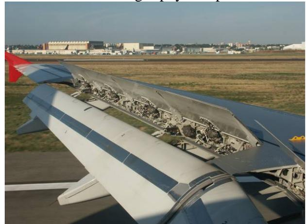
Figure1: Efficient but complex high lift system of Airbus A320
