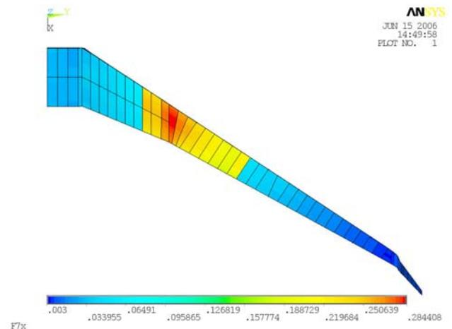
Figure 11: Wingbox thickness distribution after 2 iterations; element-wise sizing
