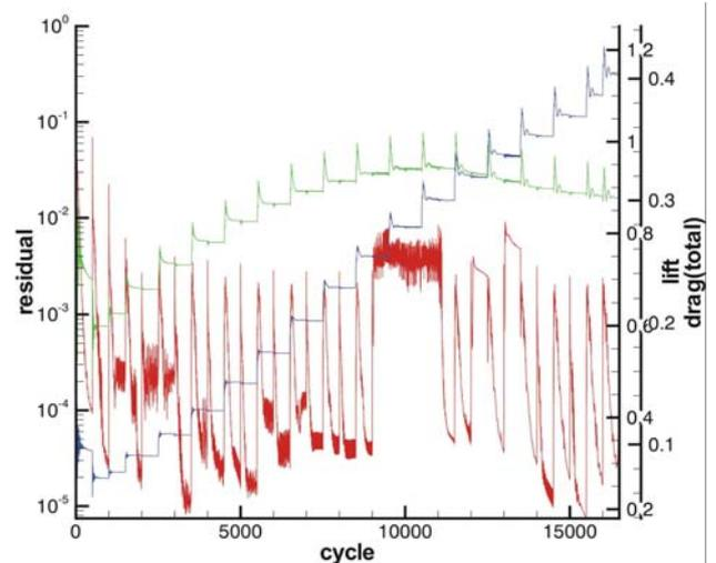
Figure 7: Residual, lift and drag coefficients of aeroelastic coupled alpha variation
