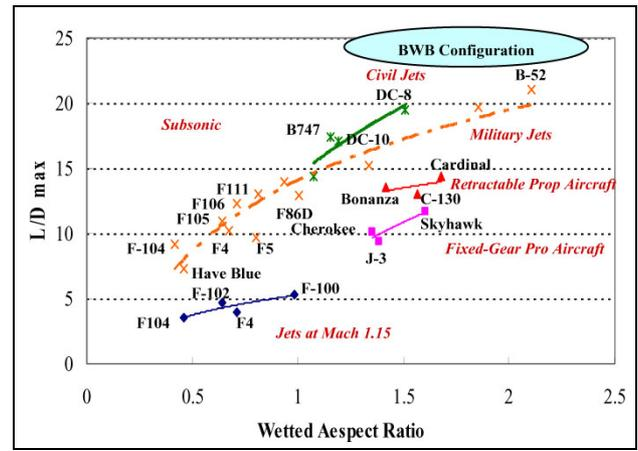
Fig. 4 L/D Estimation Chart with Wetted Aspect Ratio
