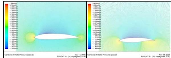
**Fig. 6** CFD Results of Body/Wing Airfoil Sections
