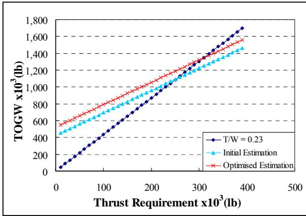
Fig. 11 Thrust Requirement vs. TOGW Diagram
