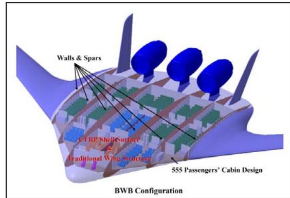
**Fig. 10** Structural BWB Conceptual Design
