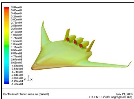
**Fig. 15** CFD Result of BWB (Pressure Contours)
