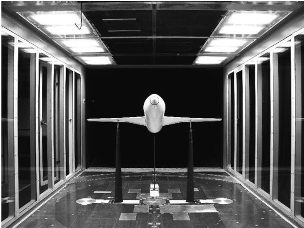
Fig. 1: Full-span configuration in the test section
