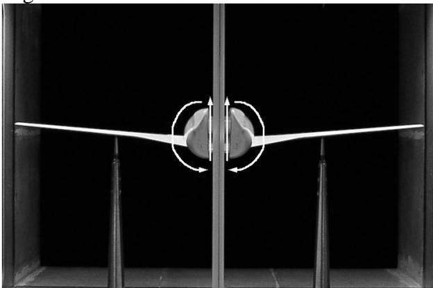
Fig. 11: Additional circulation around the fuselage
