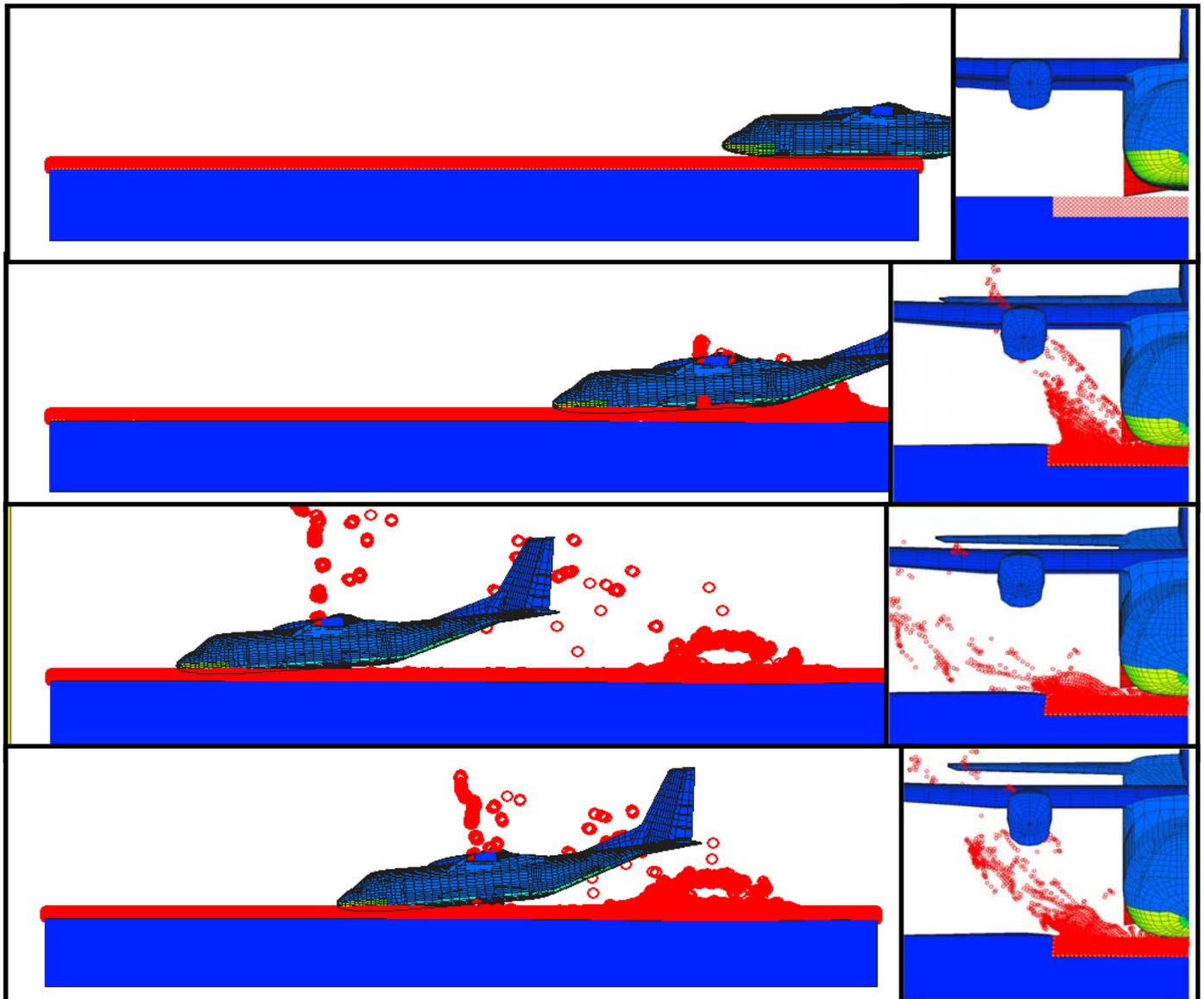
Fig. 13. EADS-CASA CN235-300M Numerical simulation considering the horizontal component of velocity and water modelled with smooth particle hydrodynamics (SPH)
