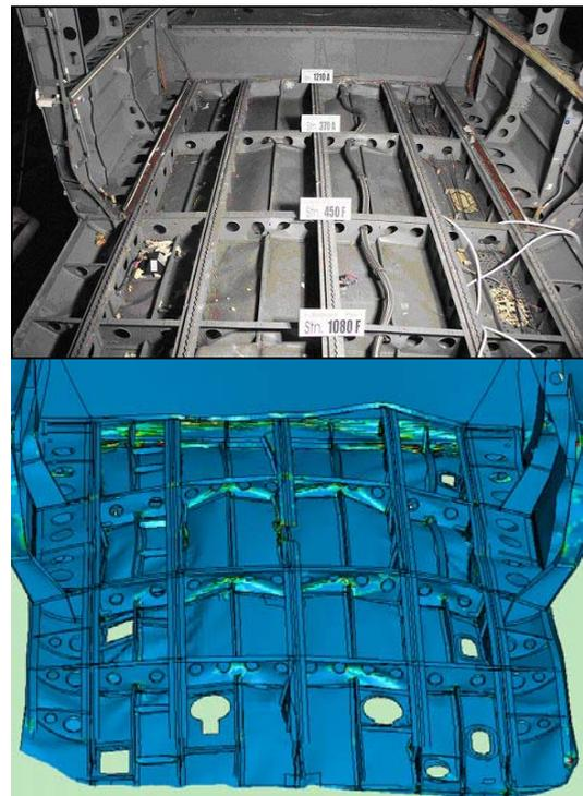
Fig. 6. Global internal view of the helicopter after removal of the floor panels, rear side (model deformation at time  $t = 80$  ms and deformation of the structure after the test), [46].
