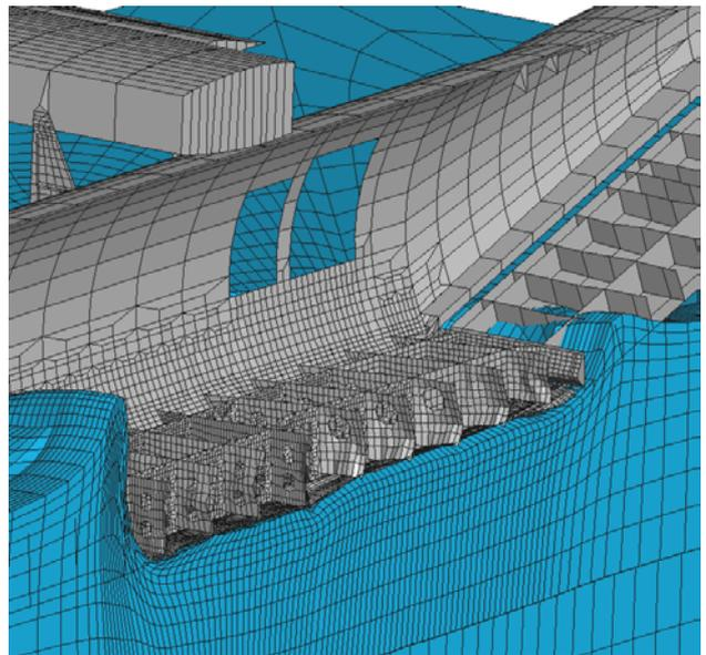
Fig. 16. Drop simulation of an A/C flexible model impacting on water, [61].
