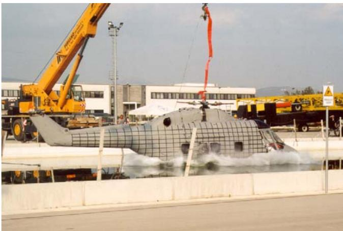
Fig. 5. WG30 Helicopter drop test, [46].
