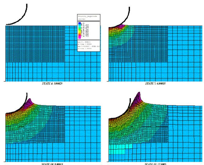
Fig. 3. Simulation of cylinder impacting on water, [46].
