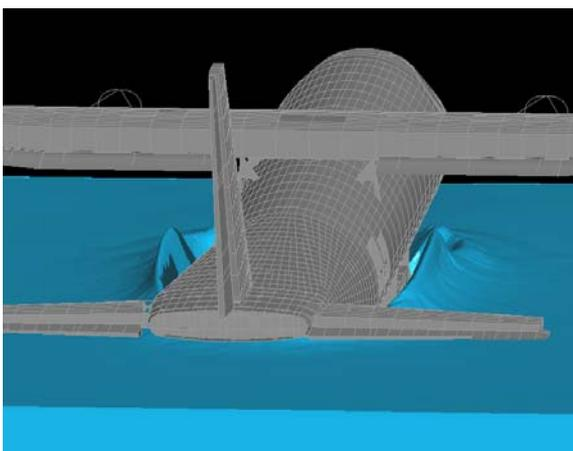
Fig. 10. EADS-CASA CN235-300M Numerical simulation. Vertical drop test, [51].
