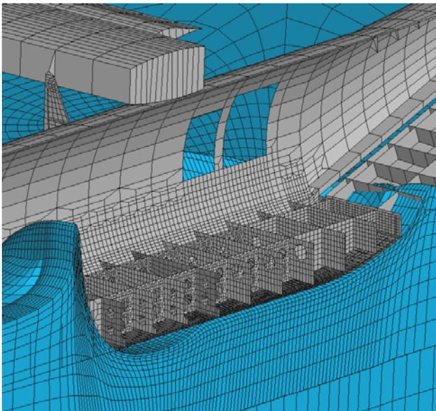
Fig. 15. Drop simulation of an A/C rigid model impacting on water, [61].
