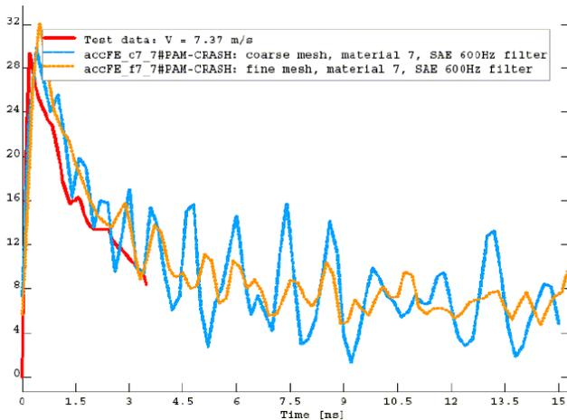
Fig. 4. Contact force time history in the cylinder impact. Test vs. Numerical simulation, [46].
