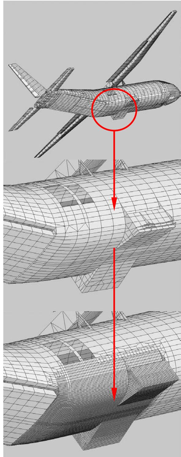
Fig. 9. EADS-CASA CN235-300M FE explicit model. Detail of refined area, [51].
