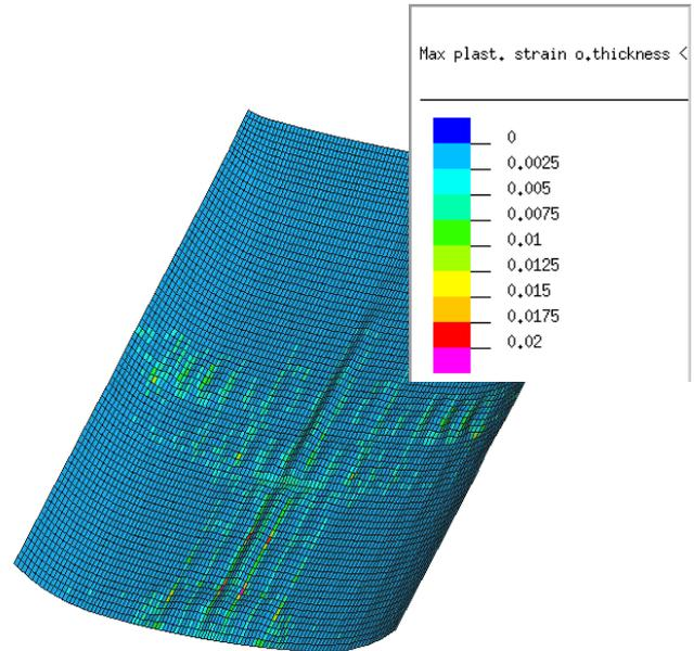
Fig. 19. Maximum and effective strain over the thickness at the skin panels[59].
