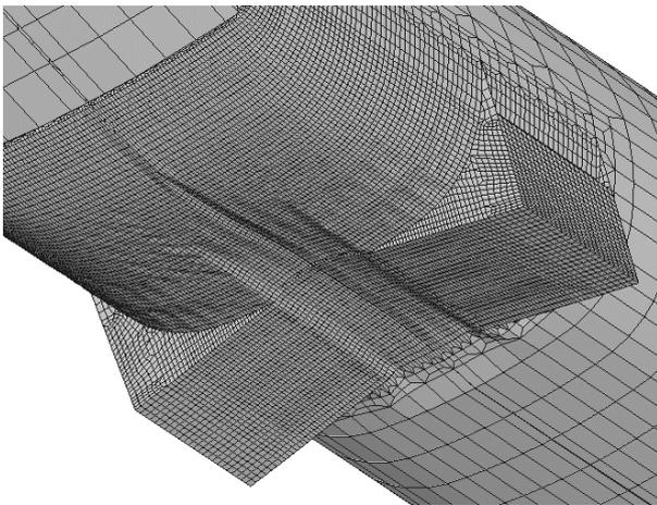
Fig. 18. Fuselage deformations under ditching loads, [59].
