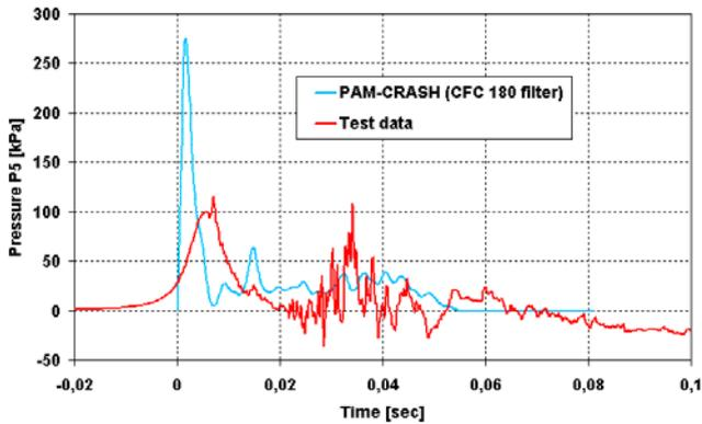
Fig. 8. Pressure time histories in WG30 drop test. Test vs. Numerical simulations, [46].
