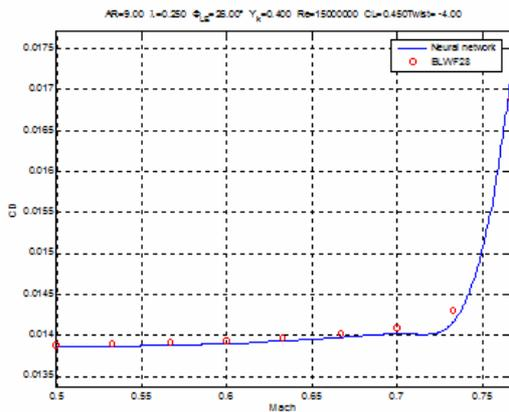
Fig. 40 – Drag divergence for a high aspect ratio twisted wing predicted by the MLP network. The twist angle for all wings is  $4^\circ$ .
