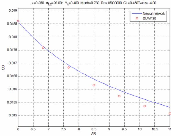
Fig. 38 –  $C_D$  prediction for wings of different aspect ratios. The twist angle for all wings is  $4^\circ$ . Comparison is made with results of a full-potential code.
