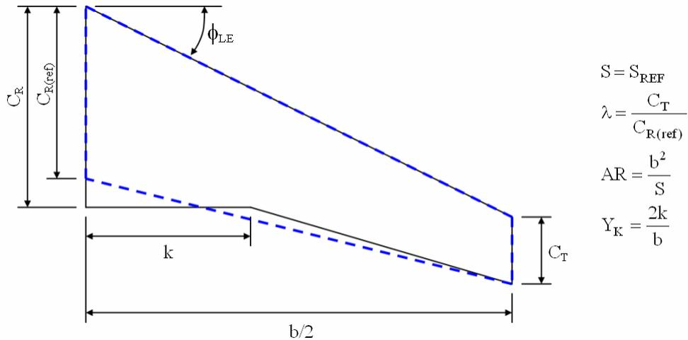
Figure 37 - Top right, the chosen parameters for the definition of the wing planform. Solid lines: actual wing; Dashed lines: reference wing (used for calculation of the taper ratio as input variable only).
