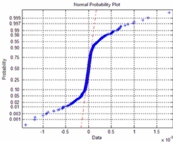
Figure 12 - NPP of residuals –  $C_D$ . Normal probability plot of residuals for the drag coefficient of the wing-body configuration.
