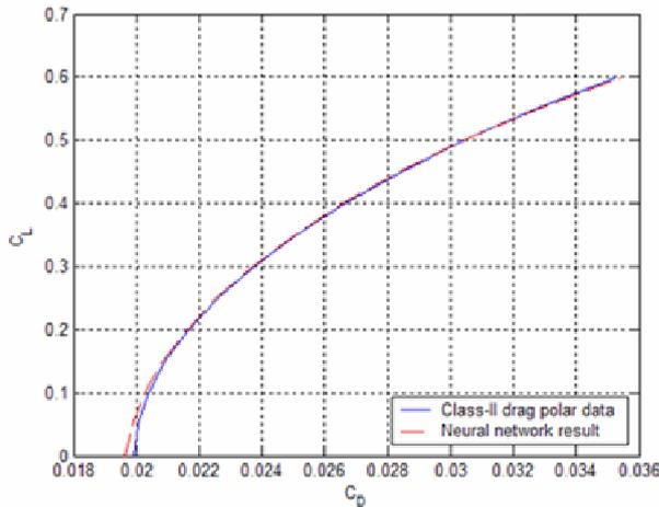
Fig. 22 - Drag polar for the regional jet test case.
