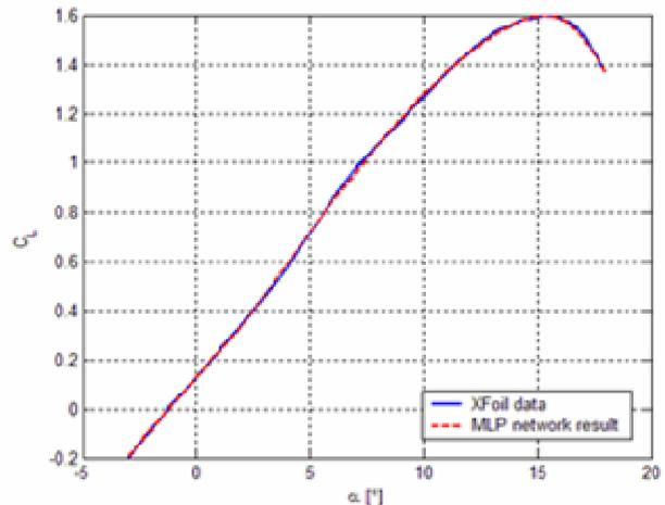
Figure 14 -  $C_l$  vs.  $\alpha$  for NACA 23012.  $Re=1.5 \times 10^6$  and Mach number of 0.20.
