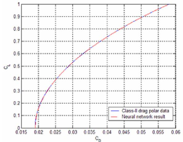
Fig. 20 - Drag polar for the regional jet test case.  $Mach$  of 0.35 and  $Re = 1.75 \times 10^7$ .
