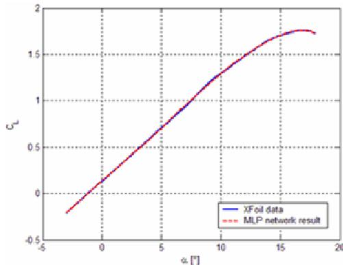
Fig. 18 -  $C_l$  vs  $\alpha$  for NACA 23012.  $Re = 4.5 \times 10^6$   $M = 0.20$ .
