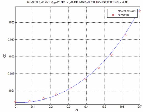
Fig. 39 – Predicted drag polar for a high-aspect ratio twisted wing. Comparison is made with results of a full-potential code.
