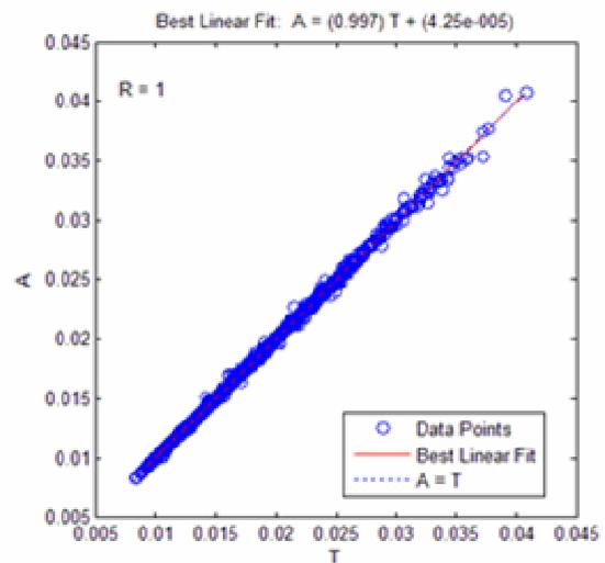
**Figure 11 - Validation fit –  $C_D$ . Comparison between expected outputs and network answers for the drag coefficient of the wing-body configuration.**
