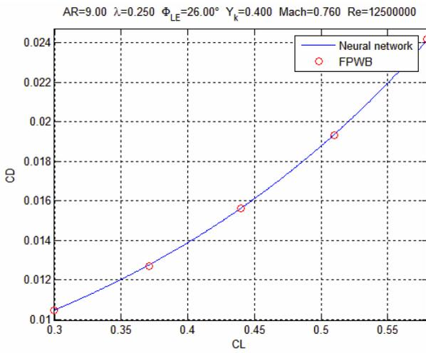
Fig. 27 - Drag polar for a typical wing-body configuration.
