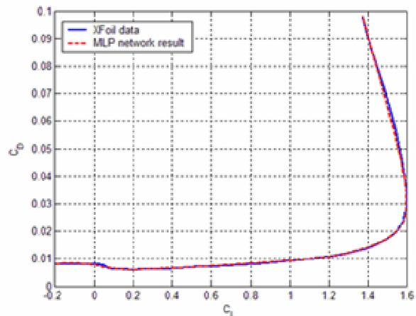
Fig. 15 -  $C_d$  vs.  $C_l$  for NACA 23012.  $Re = 1.5 \times 10^6$ , Mach = 0.20, natural BL transition.
