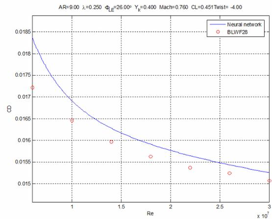
Fig. 41 – Predicted drag polar for a high-aspect ratio twisted wing.
