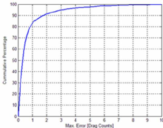
Figure 13 - Cumulative probability of errors –  $C_D$ . Percentage of points with error smaller or equal than a threshold for the wing-body configuration.
