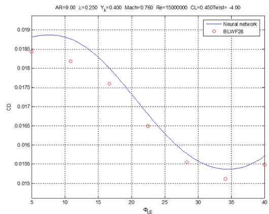
Fig. 43 -  $C_D$  variation with leading-edge sweepback angle. AR = 9, Mach = 0.70, Re =  $2 \times 10^7$ .
