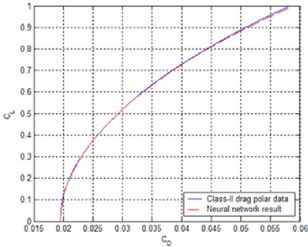
Fig. 21 - Drag polar for the regional jet test case.
