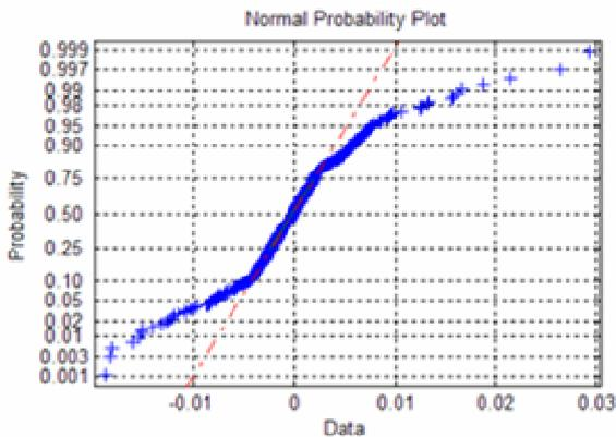
**Fig. 6 - NPP of residuals –  $C_l$ . Normal probability plot of residuals for the lift coefficient of NACA23012 airfoil.**
