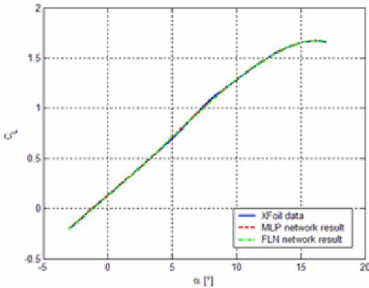
Figure 16.  $C_l$  vs  $\alpha$  for NACA 23012.  $Re = 2.5 \times 10^6$  and  $Mach = 0.20$ .
