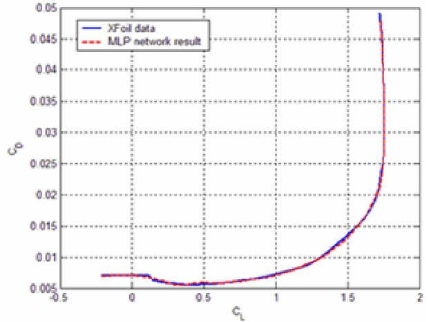
Fig. 19 -  $C_d$  vs.  $C_l$  for NACA 23012 .  $Re=4.5 \times 10^6$ ,  $Mach = 0.20$ , natural BL transition.
