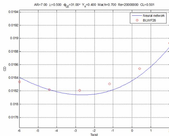
Fig. 42 -  $C_D$  variation with wing twist. AR = 7, Mach = 0.70, Re =  $2 \times 10^7$ .
