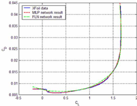
Fig. 17 –  $C_d$  vs.  $C_l$  for NACA23012.  $Re = 2.5 \times 10^6$ ,  $Mach = 0.20$ , and natural BL transition.
