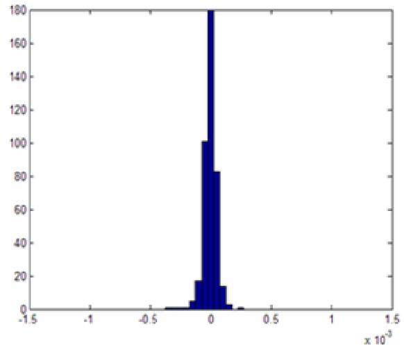
**Fig. 8 - Histogram of residuals –  $C_d$ . Histogram of residuals for the drag coefficient of NACA23012 airfoil.**
