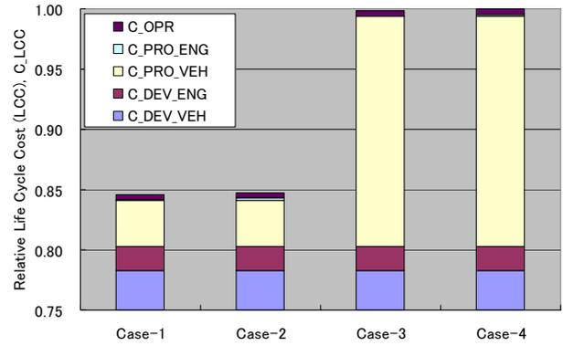
**Fig.5. Relative Life-cycle-cost Comparison of LE-7 based TYPE-R Case Studies (5LpA)**
