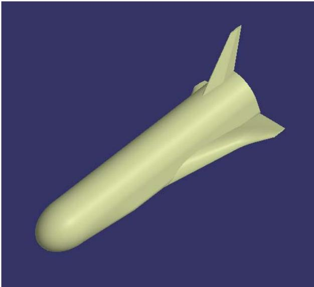
Fig.4. TYPE-R Vehicle (SSTO/VTHL: Vertical Takeoff and Horizontal Landing)
