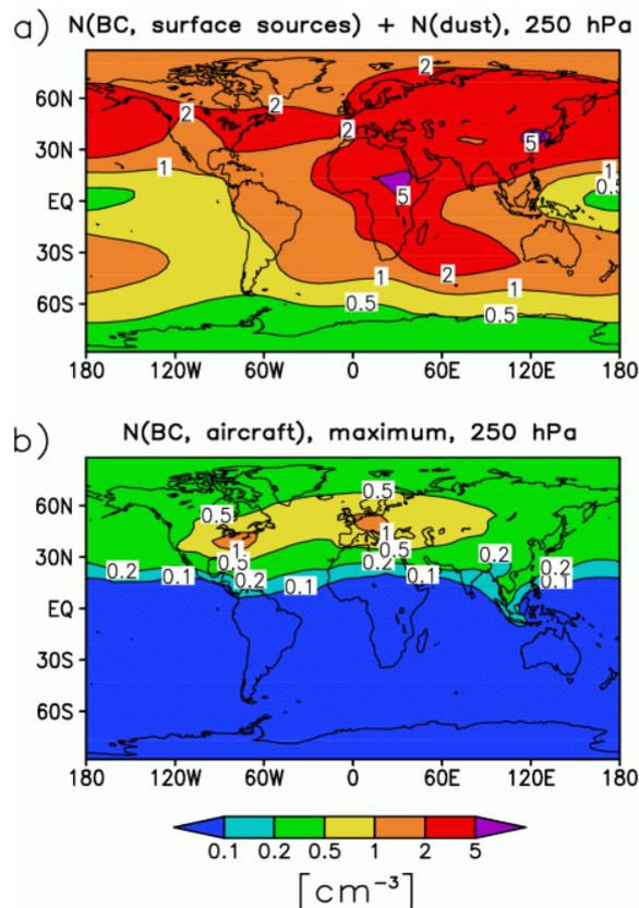
Fig. 1. Annual mean number concentrations [particles/cm<sup>3</sup>] of potential IN at 250 hPa (within main aircraft flight level; approximately at 10 km altitude). (a) Mineral dust and hydrophilic BC particles originating from surface sources. (b) BC particles from aircraft (maximum estimate [4]). The Figure is adopted from a previous publication [6].
