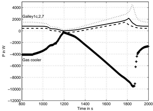
**Fig. 10** Heat flow rate at the evaporator and gas cooler (ambient temperature change at the gas cooler)
