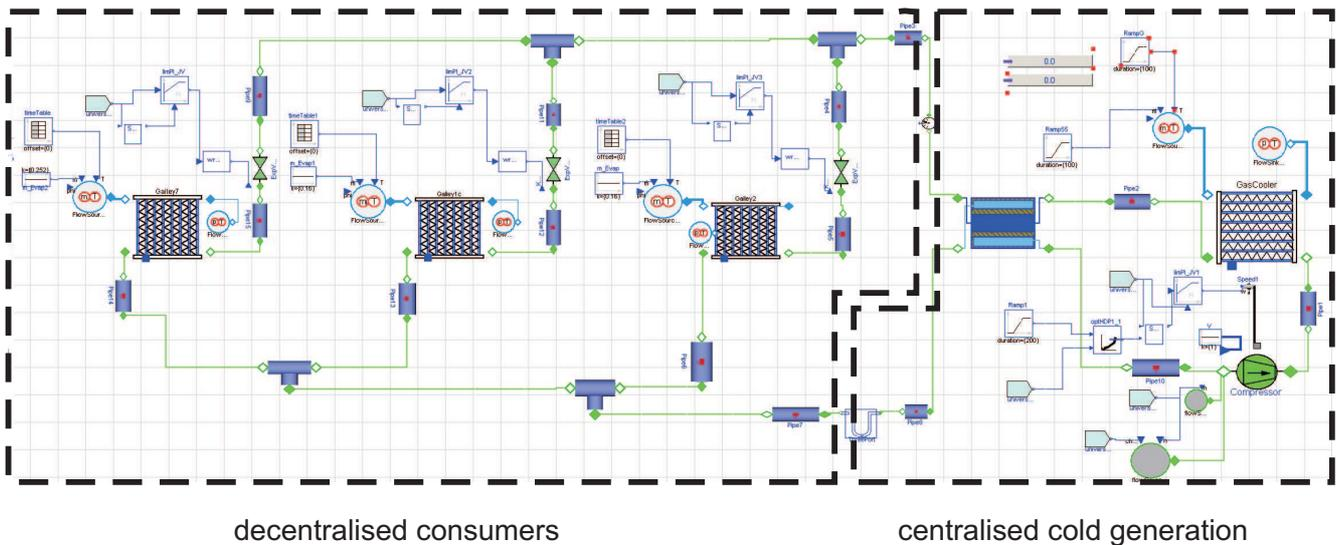
**Fig. 3** Dymola/Modelica model of a three consumer direct evaporating CO2 system
