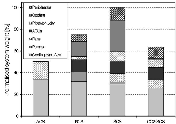
Fig. 2 Weight estimation for on-board cooling systems
