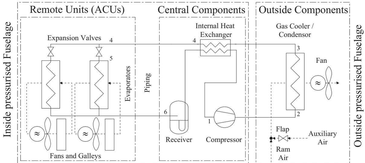
Fig. 1 CO<sub>2</sub> direct evaporating system
