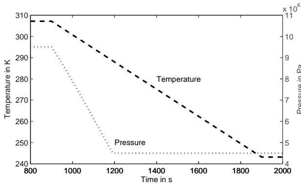
**Fig. 6** Air temperature at the gas cooler and high pressure change
