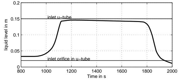
**Fig. 8** Liquid level in the receiver (ambient temperature change at the gas cooler)
