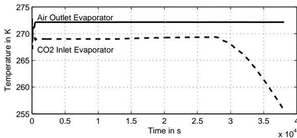
**Fig. 16** Temperature at the evaporator, emptying process
