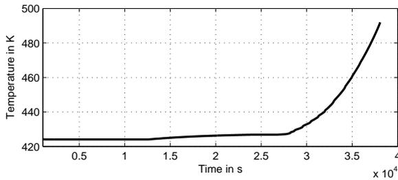
**Fig. 15** Compressor discharge temperature, emptying process
