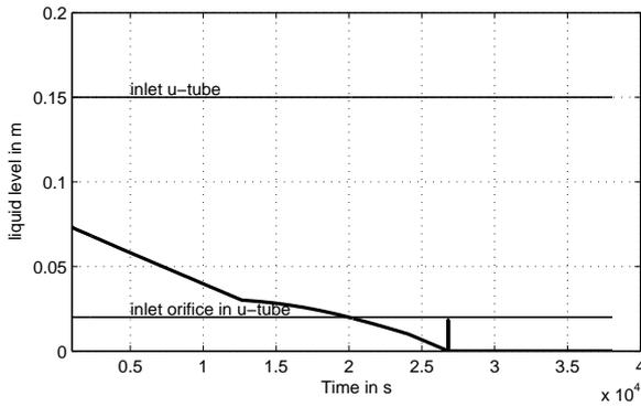
**Fig. 14** Liquid level in the receiver, emptying process
