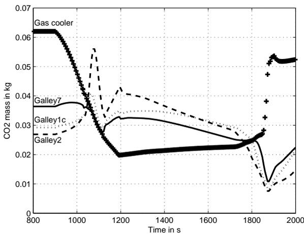
**Fig. 7** CO<sub>2</sub> mass in the main components (ambient temperature change at the gas cooler)
