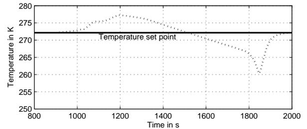
**Fig. 9** Air outlet temperature at an evaporator (ambient temperature change at the gas cooler)
