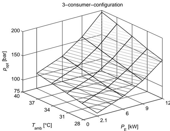
Fig. 4 Optimal pressure for the 3 consumer configuration
