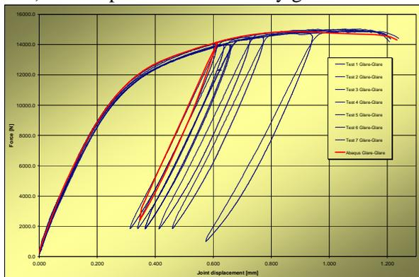
Figure 16. Rivet strength test data.
