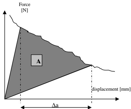
Figure 8. Schematic presentation of the determination of the fracture energy  $A$ .
