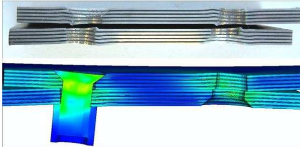
Figure 15. Cross sections of failed riveted joints: experiment (top), numerical (bottom)
