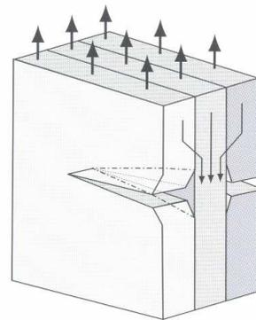
Figure 4. Fiber bridging in FML.
