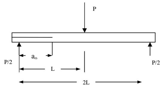
Figure 9. Test (top) and specimen geometry for the Mode II test.
