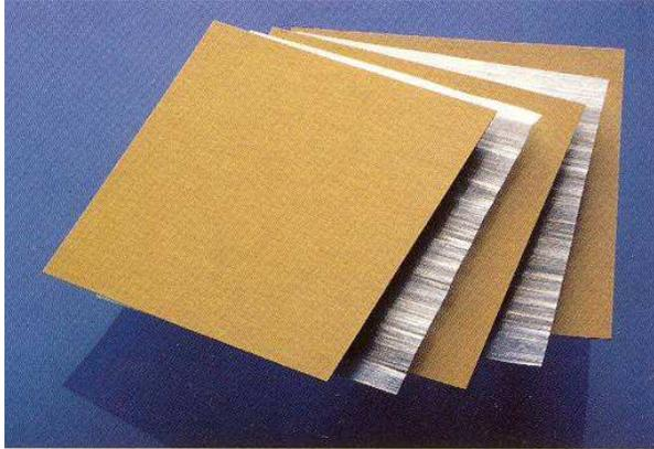
Figure 1. Example of a FML (GLARE 2-3/2-0.4)
