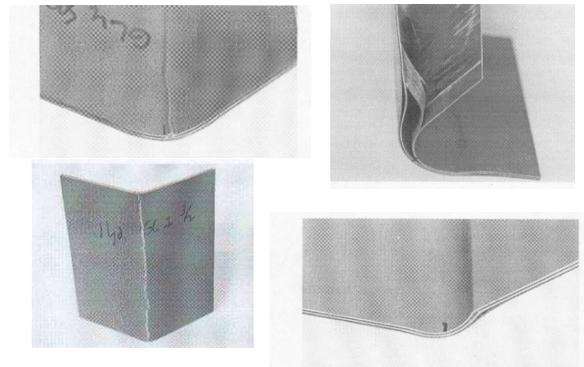
*Figure 5. Some basic failure modes of FML. (clockwise starting at top-left: buckling of a metal layer, edge delamination, delamination close to a bend zone, cracking of metal layer).*
