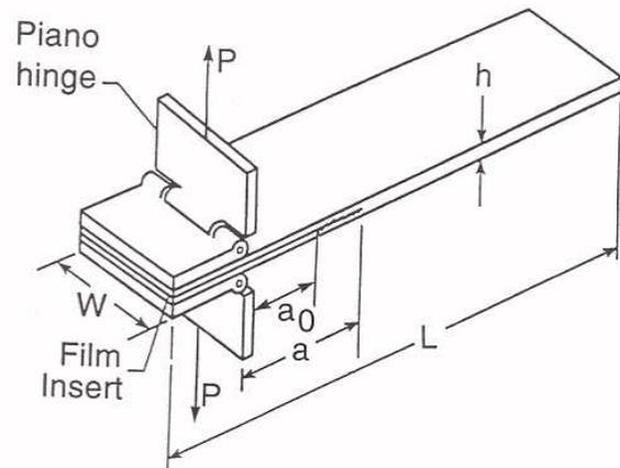
Figure 7: Test (top) and test specimen (bottom) for Mode I testing.
