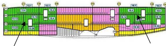
Figure 3. GLARE-panels in the Airbus A380
