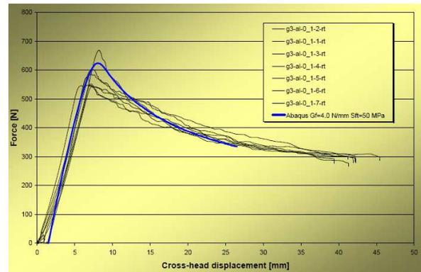
Figure 13. Test and numerical results for Mode I Fracture Energy testing of GLARE-3 at RT.
