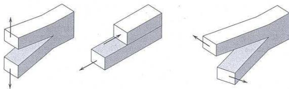
Figure 6. The three principal fracture types: Mode I, Mode II and Mode III. (from left to right).
