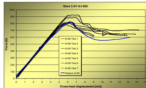
Figure 14. Test and numerical results for Mixed Mode Fracture Energy testing of GLARE-3 at 80°C.
