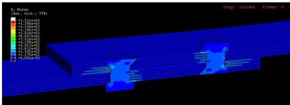
Figure 12. FE model of a riveted lap joint.
