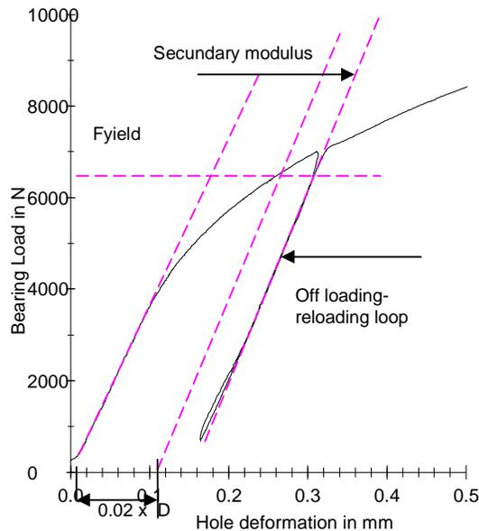
Figure 11. The cycle to determine the bearing yield strength.
