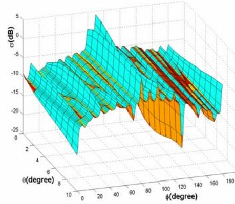
Fig. 5 The RCS Approximation Model using Kriging Method
