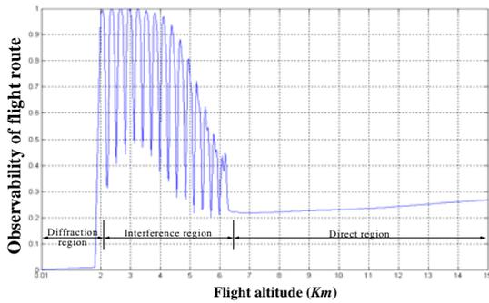
Fig. 6 Observability of Flight Route vs Flight Altitude
