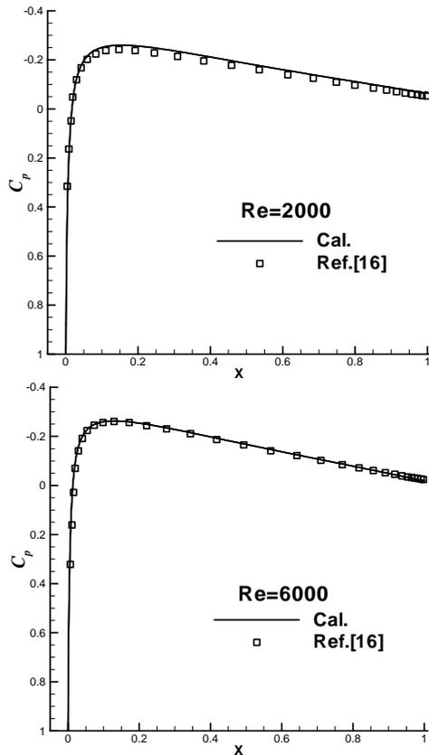
Fig.2. Comparison of computed pressure distribution with references over NACA 0008 airfoil ( $\alpha = 0^\circ$ ) at low Reynolds numbers
