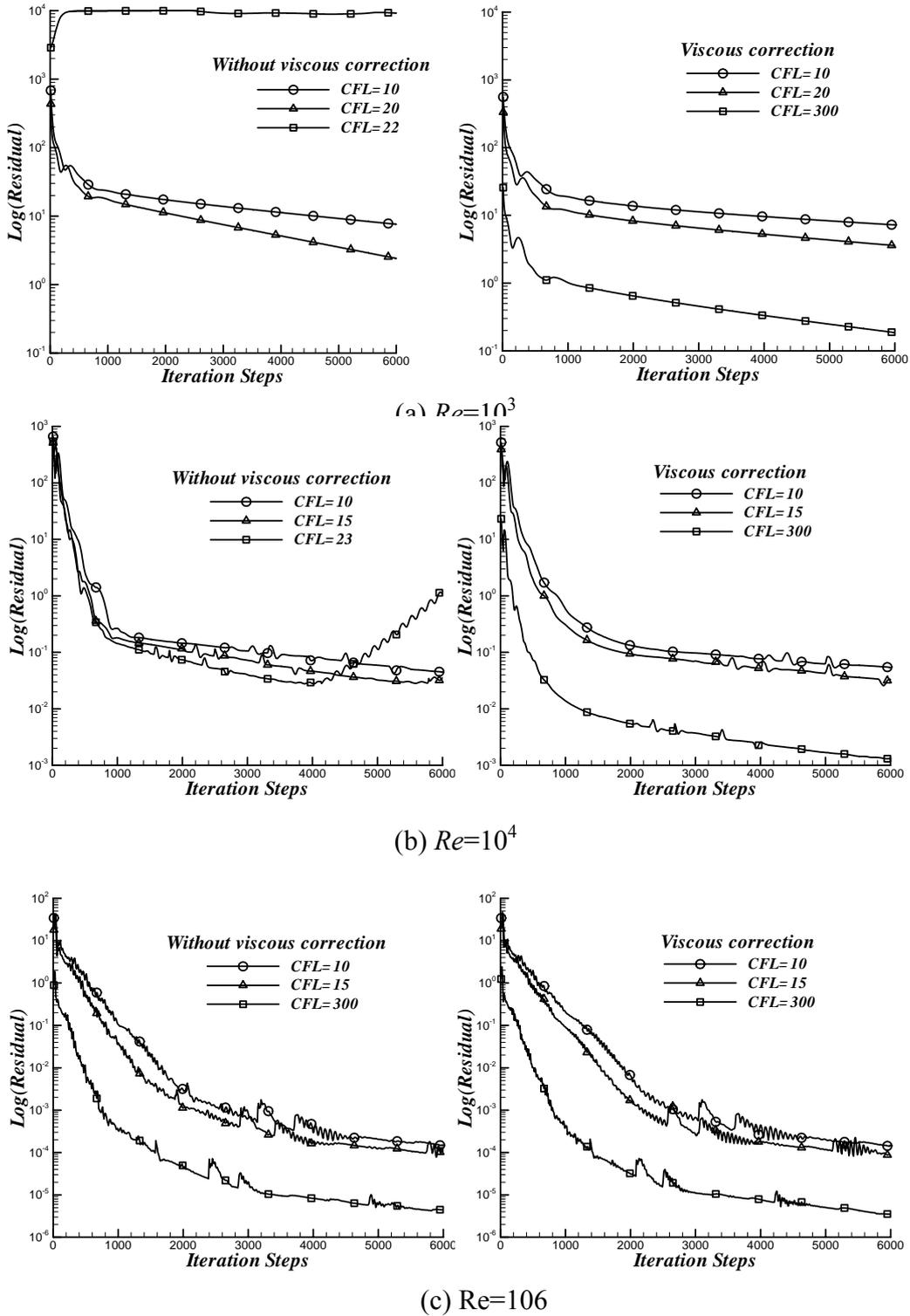
Fig.3. Stability and efficiency of LU-SGS method for NACA0012 airfoil at different Reynolds numbers with  $\beta = 3, \alpha = 0^\circ$
