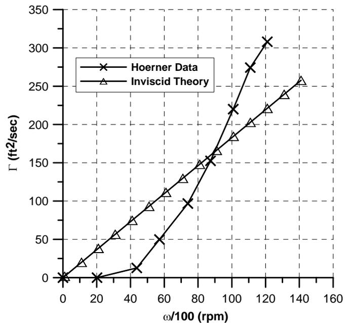
Fig. 4: Comparison of Potential and Experimental Circulation Values vs. Rotational Velocity
