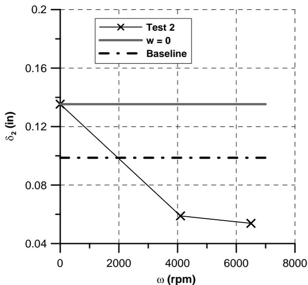
Fig. 12: Momentum Thickness Reduction vs. Rotational Velocity,  $\omega$
