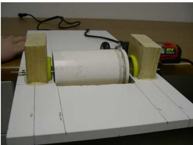
Fig. 7: Experimental Boundary Layer Control Setup
