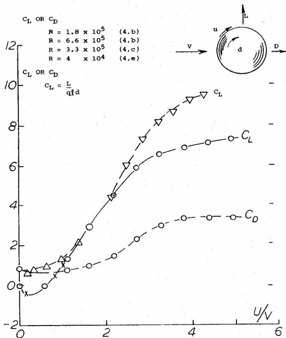
Fig. 3: Lift Generated by a Rotating Cylinder in Uniform Flow [12]
