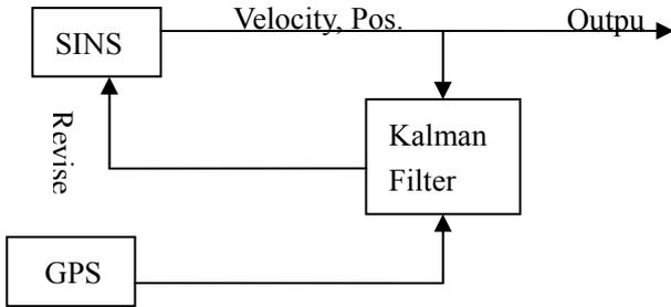
Fig.2 Closed loop GPS/SINS system
