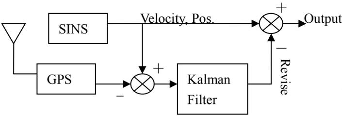
Fig.1 open loop GPS/SINS system
