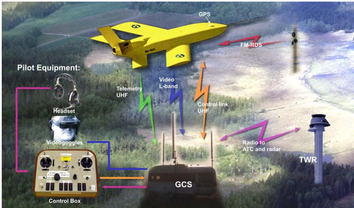
Fig. 7 – Overall view of the communication and control system
