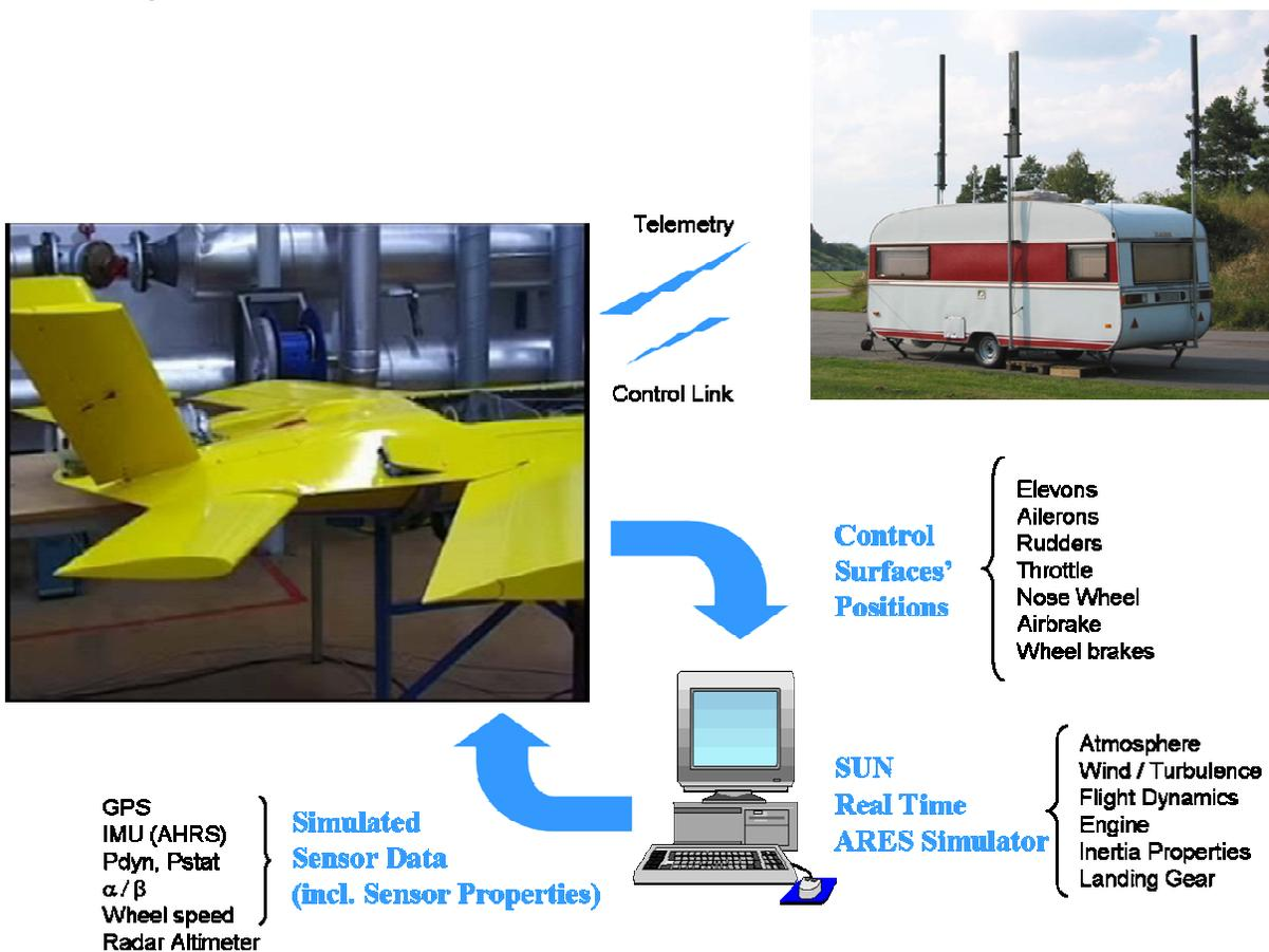
Fig. 5 – Setup of the Hardware in the Loop Simulator
