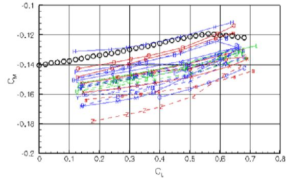
Fig. 8. DLR-F6 wing-body pitching moment results from DPW 2.
