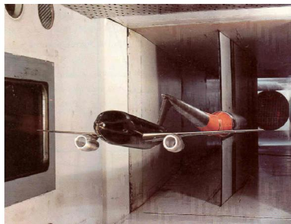
Fig. 3. DLR-F6 model in ONERA S2MA wind tunnel.
