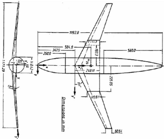
Fig. 1. DLR-F4 wing-body geometry.
