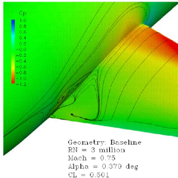
Fig. 11. RANS computed streamlines of DLR-F6 showing flow separation region.
