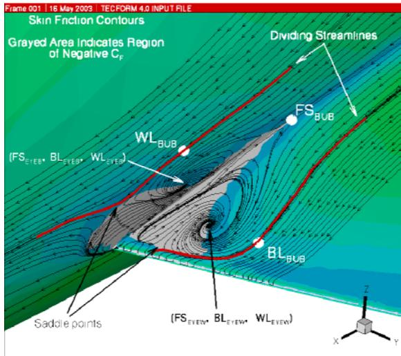
Fig. 6. RANS code predicted DLR-F6 inboard wing separation bubble, definition of measurement points.
