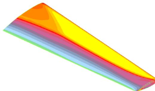
Fig. 13. RANS computed pressure contours of DPW-W1 at Mach 0.76.
