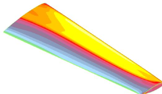
Fig. 14. RANS computed pressure contours of DPW-W2 at Mach 0.76.
