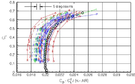
Fig. 9. DLR-F6 wing-body drag polar results from DPW 2.
