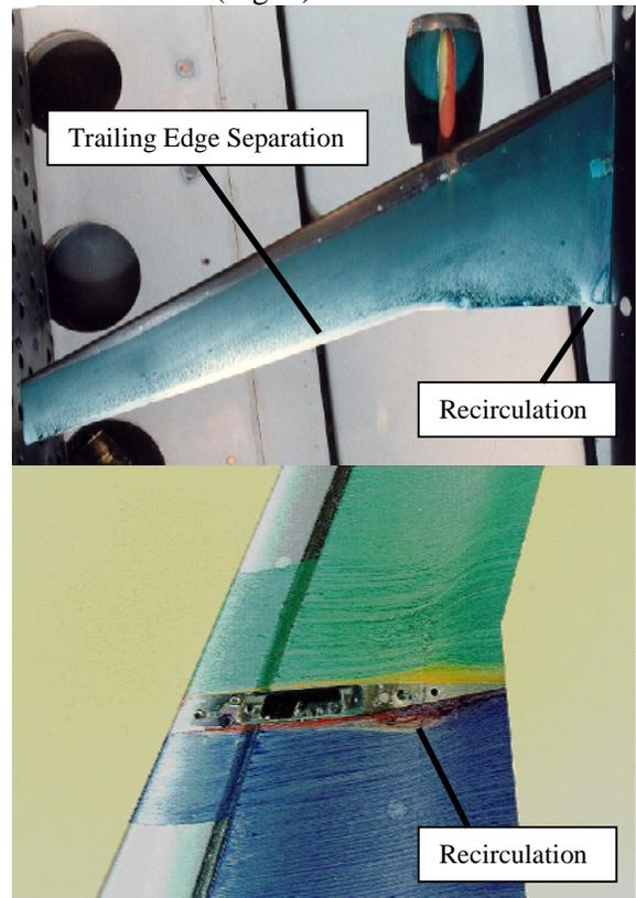
Fig. 5. DLR-F6 wind tunnel model with oil flow patterns.
