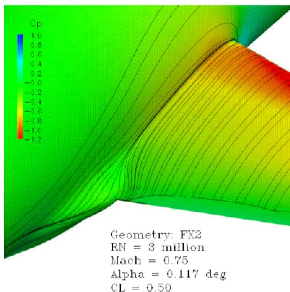
Fig. 12. RANS computed streamlines of DLR-F6 with FX2 fairing showing elimination of the flow separation region.
