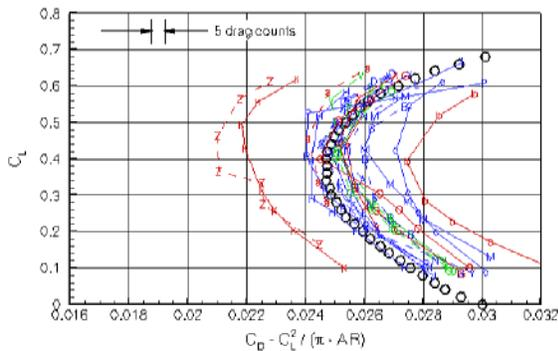
Fig. 10. DLR-F6 wing-body-pylon-nacelle drag polar results from DPW 2.
