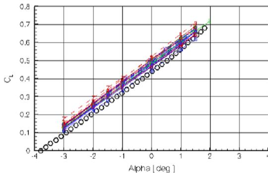
Fig. 7. DLR-F6 wing-body lift curve results from DPW 2.
