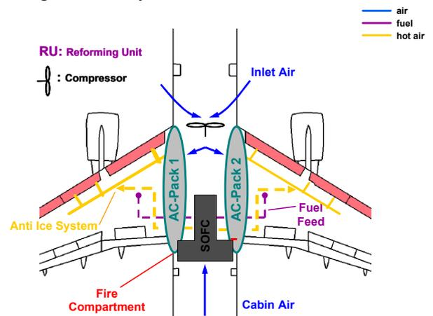
Fig. 13. Concept 3: SOFC in Aircraft Center
