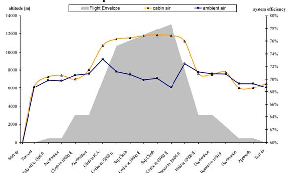
Fig. 3. SOFC System Performance
