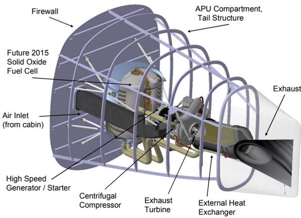
Fig. 5. SOFC System Pre-Design
