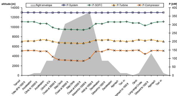
Fig. 4. SOFC System Component Powers
