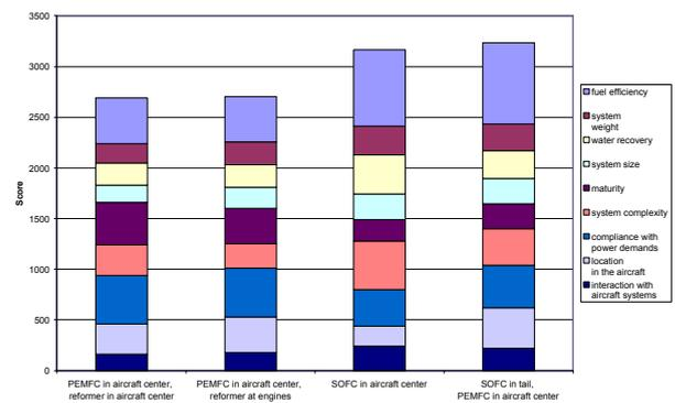
Fig. 15. Weighted Score of Fuel Cell Systems
