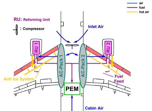
Fig. 12. Concept 2: PEMFC in Aircraft Center, Reformer at Engines
