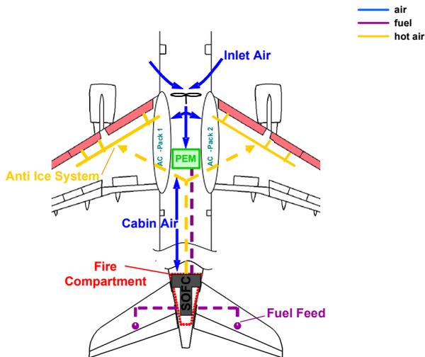
Fig. 14. Concept 4: SOFC in Aircraft Tail, PEMFC in Aircraft Center
