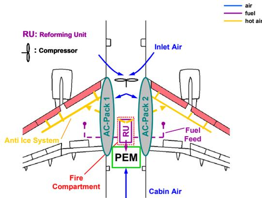
Fig. 11. Concept 1: PEMFC in Aircraft Center
