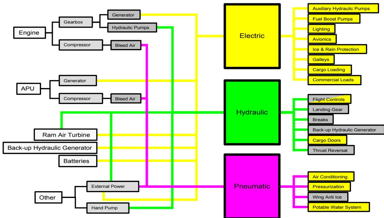
Fig. 1. Energy Supply (left) and Consumers (right) with Future Electric Systems (yellow) According to the Scenario
