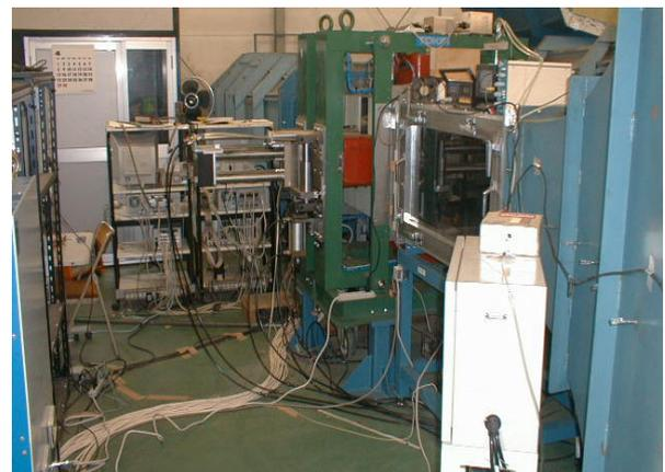
Fig.14. Test Section and the JAXA 60cm MSBS
