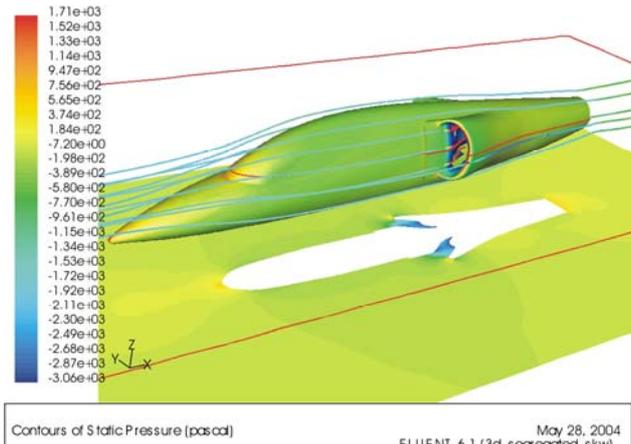
Fig. 10. Calculated static pressure distribution in the flow field around the fuselage with running engine at flight velocity  $v = 40$  m/s
