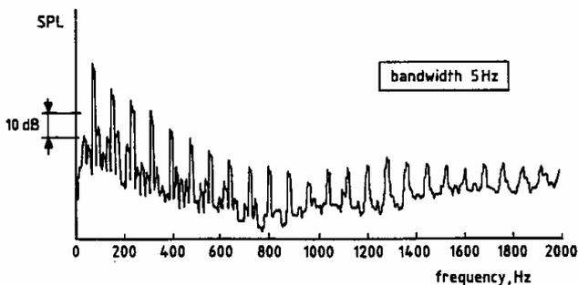
Figure 5. Spectrum of Frequencies of Cessna 150 Aircraft Noise magnitude of frequency as a result of propeller blade rotation,  $f_1$ , is expressed with :
