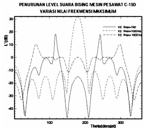
Figure 6. The result of reduction of C-150 aircraft propeller noise
