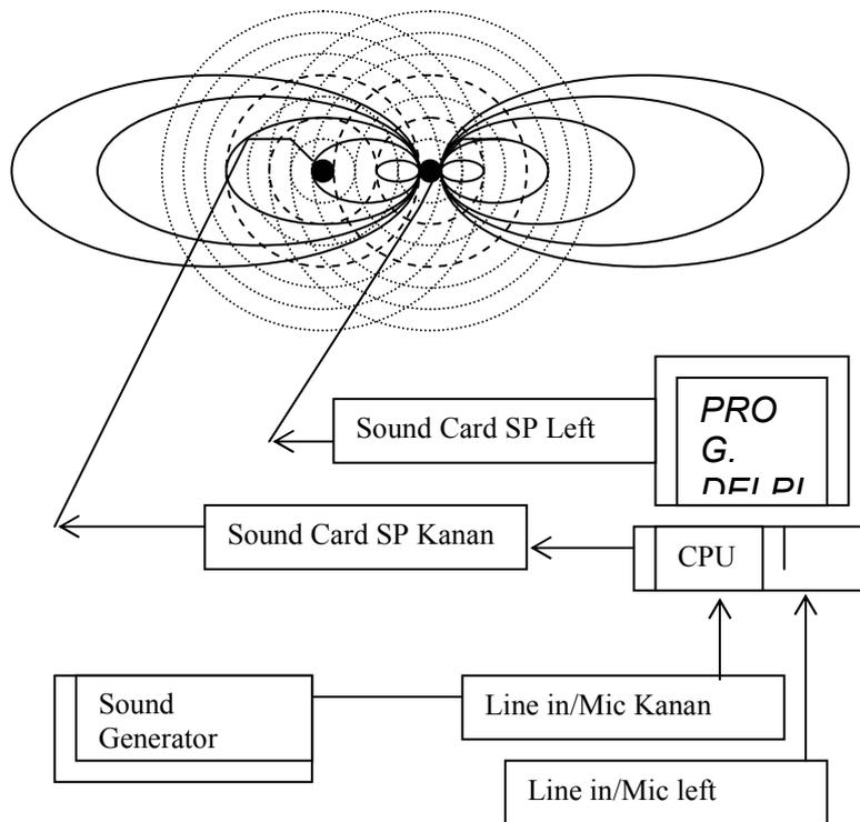
Figure 10 the schema to implementation the active noise control using multipole secondary source.
