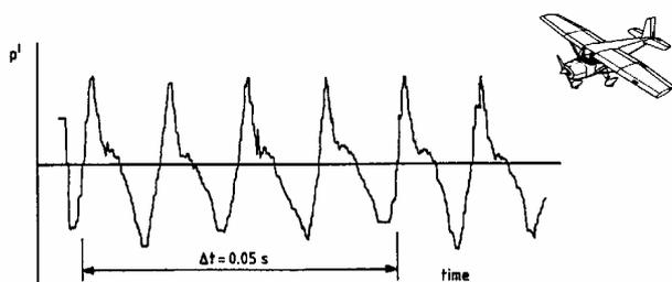
Figure 4. Picture of C-150 aircraft and diagram of time response of aircraft noise
