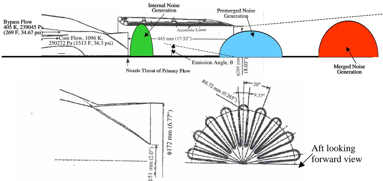
Figure 1. Side and forward views of an 18-lobed axisymmetric scale model mixer-ejector.
