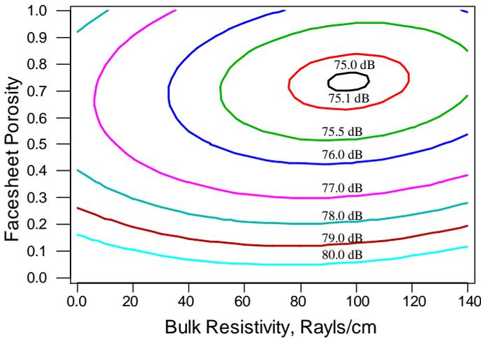
Figure 10. Contour plots for internal EPNL, Fixed Liner Parameters: Depth= $0.40''$  Facesheet Hole Diameter  $d=0.02''$ , Facesheet Thickness= $0.01''$ .
