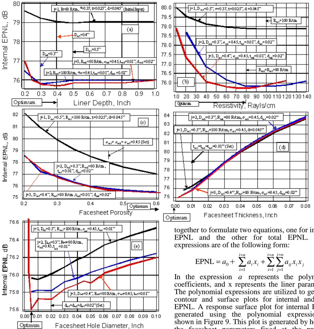
Figure 7. Iterative optimization of liner parameters. parameters. These expressions will be useful in the detailed design of the ESPR program to conduct trade studies. All the data for different liner designs generated from the iterative optimization process, plus additional data to cover the range of parameters available during the detailed design phase, are put
