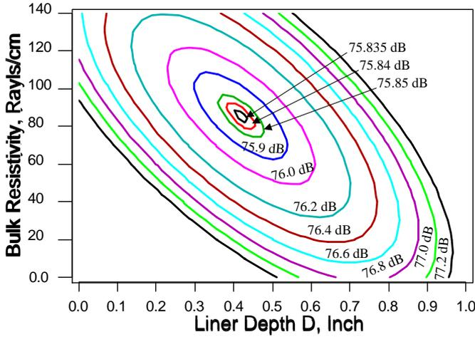
Figure 9. Contour plots for internal EPNL, Fixed Facesheet Parameters: Hole Diameter  $d=0.02''$ , Thickness= $0.01''$ , Porosity= $0.45$ .
