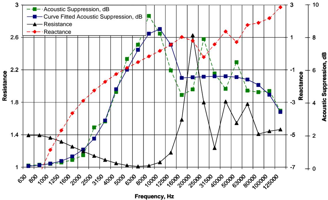
Figure 4. Predicted normal impedance spectra for the liner used in the axisymmetric ejector and the predicted acoustic suppression spectrum,  $R=12.5$  Rayls/cm,  $D=0.4''$ ,  $\sigma=37\%$ ,  $t=0.025''$ ,  $d=0.045''$ ,  $T=1008^\circ R$ ,  $M=0.65$ ,  $OASPL=166$  dB,  $M_x=0.75$ ,  $T_x=1467^\circ R$
