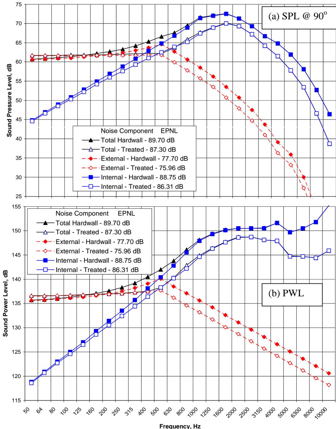
Figure 3. Total and extracted external and internal (a) SPL and (b) PWL spectra for scale model mixer-ejector for hardwall and treated configurations for an arbitrary ejector treatment, Sideline distance=1774.4 ft.,  $A_8=2505 \text{ in}^2$ ,  $\text{NPR}=2.5$ ,  $T_1=1512^\circ\text{R}$ ,  $M_F=0.3$ .
