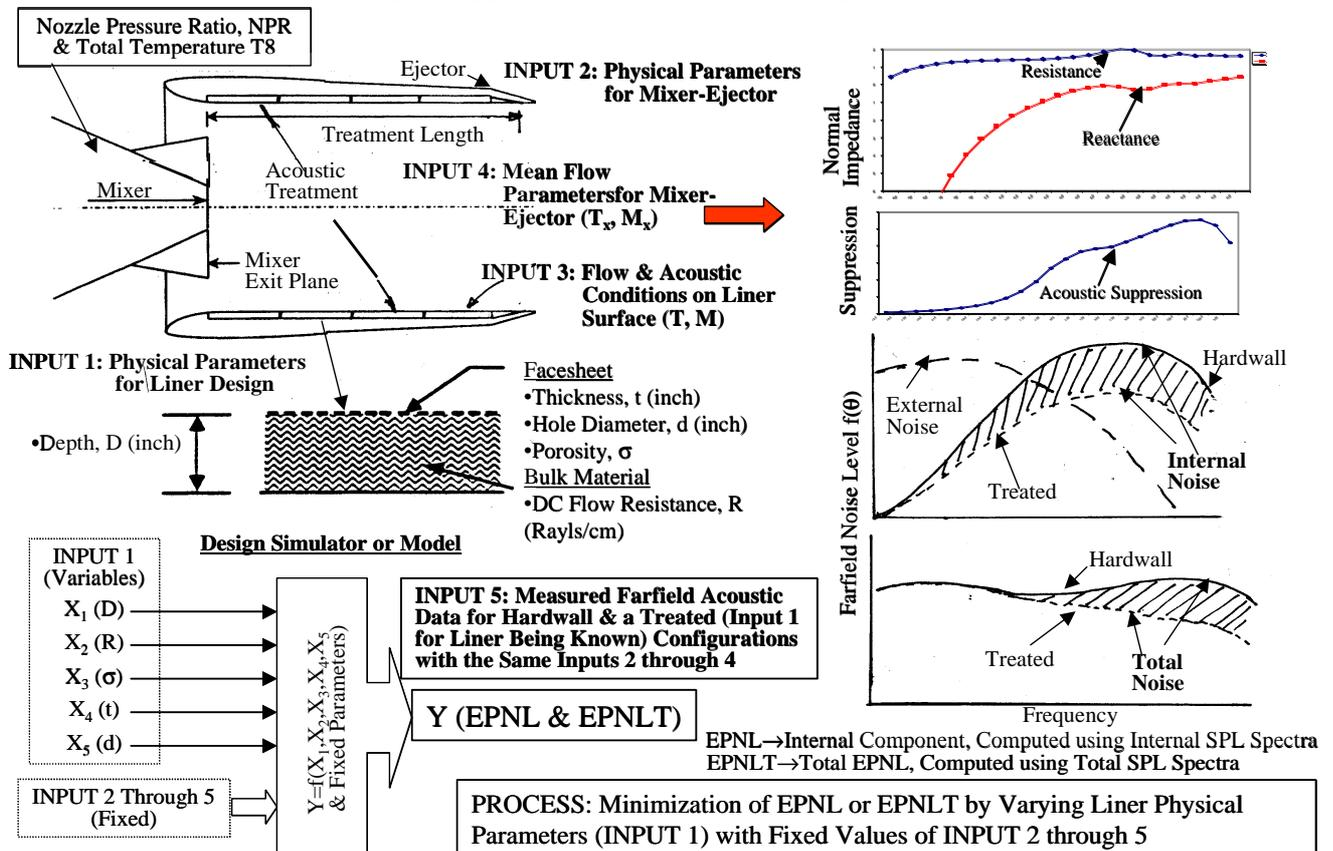
Figure 2. Process of estimating farfield noise due to acoustically treated ejector
