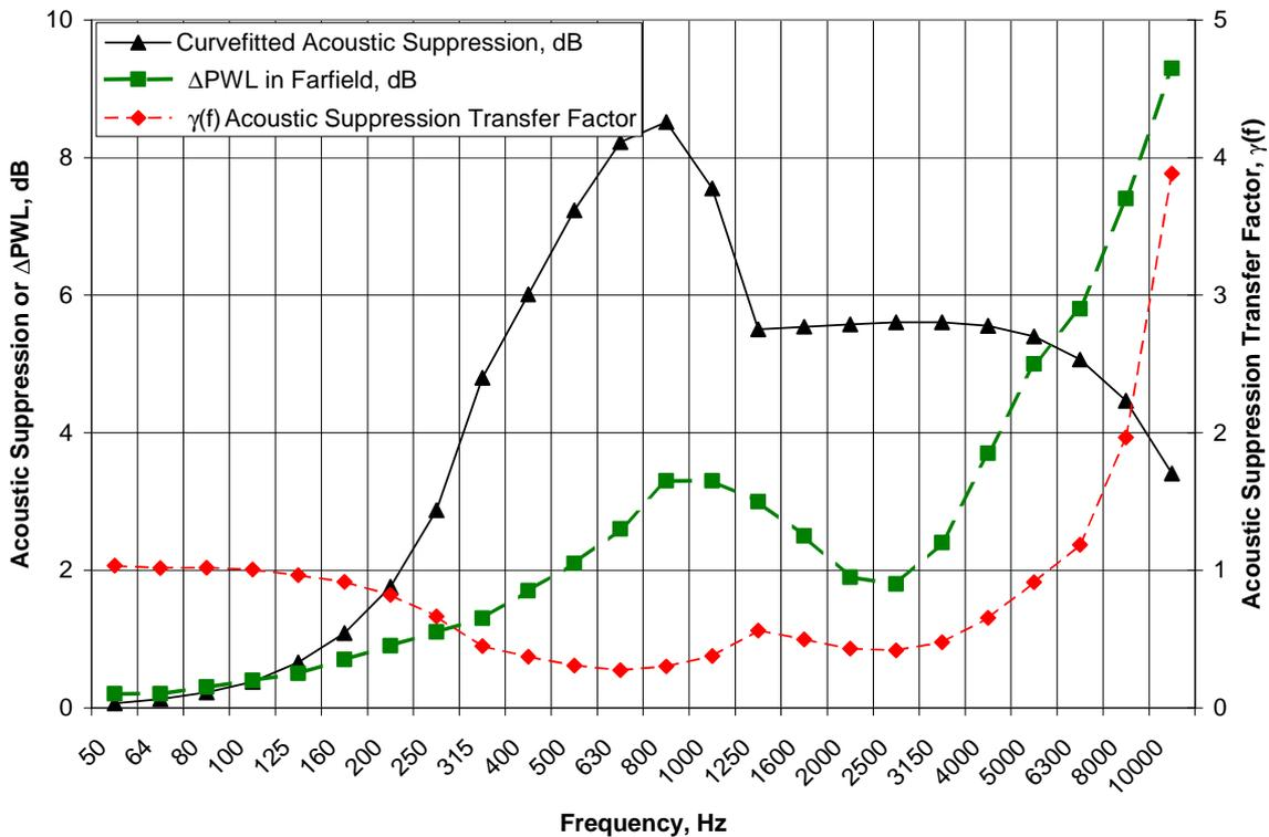
Figure 5. Predicted acoustic suppression, computed  $\Delta PWL$  and linear frequency factor  $\gamma(f)$  for the liner used in the axisymmetric ejector,  $R=12.5$  Rayls/cm,  $D=0.4''$ ,  $\sigma=37\%$ ,  $t=0.025''$ ,  $d=0.045''$ ,  $T=1008^\circ R$ ,  $M=0.65$ ,  $OASPL=166$  dB,  $M_x=0.75$ ,  $T_x=1467^\circ R$
