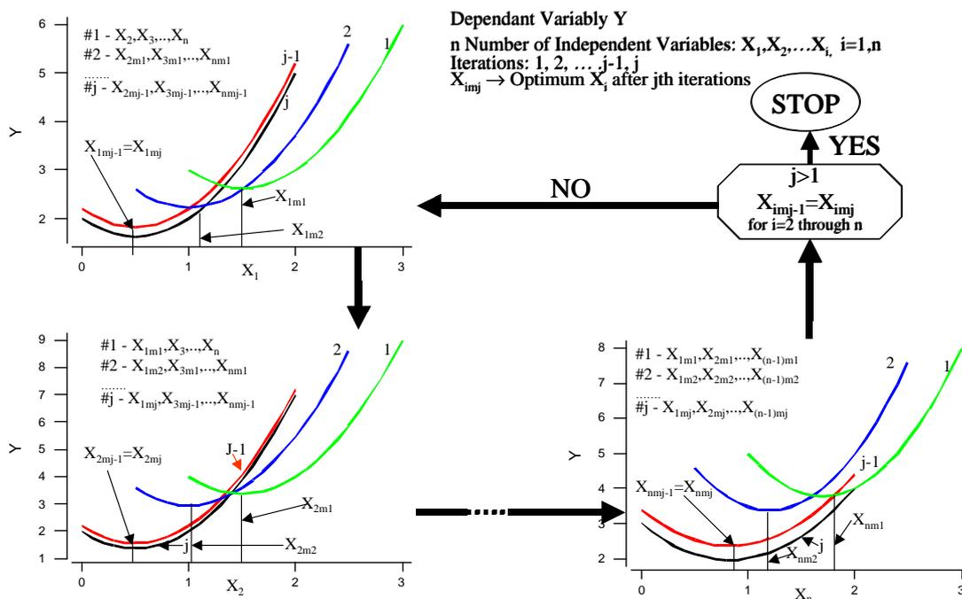
Figure 6. Process map for an iteration procedure for liner design optimization.
