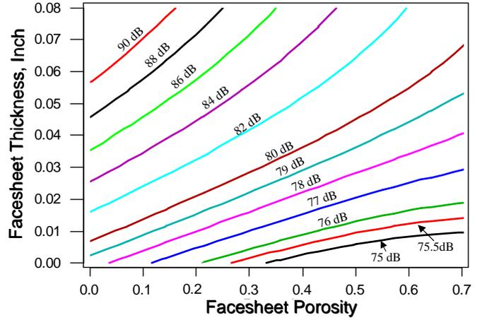
Figure 11. Contour plots for internal EPNL, Fixed Liner Parameters: Depth= $0.40''$  Bulk Resistivity= $80$  Rayls/cm, Facesheet Hole Diameter  $d=0.02''$ .
