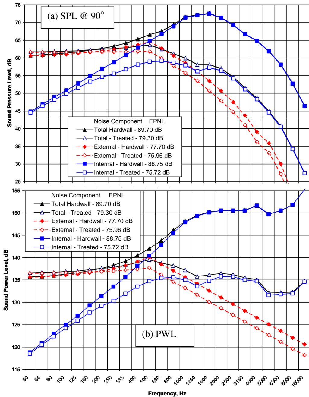
Figure 8. Total and extracted external and internal (a) SPL and (b) PWL spectra for scale model mixer-ejector for hardwall and optimally treated configurations, Sideline distance=1774.4 ft.,  $A_8=2505 \text{ in}^2$ ,  $\text{NPR}=2.5$ ,  $T_t=1512^\circ\text{R}$ ,  $M_F=0.3$ .
