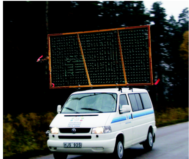
Fig. 1 Tufting grid mounted on vehicle
