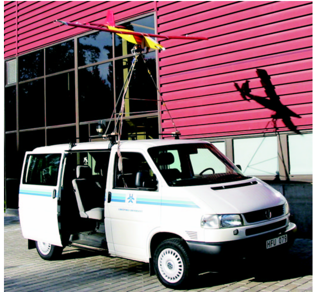
Fig. 5 Captive carry rig and test vehicle
