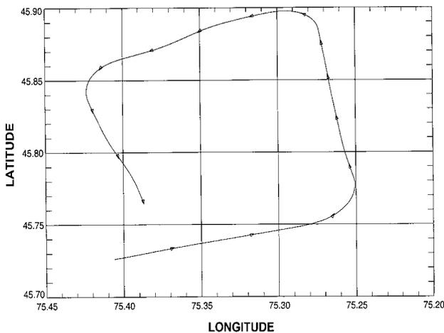
Figure 2: Wind Box Manoeuvre
