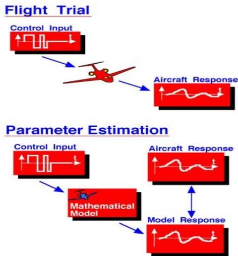
Figure 3: Aero. Model Identification Concept
