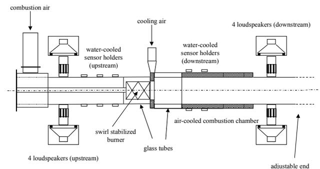
**Fig. 1** Schematic of the atmospheric test facility
