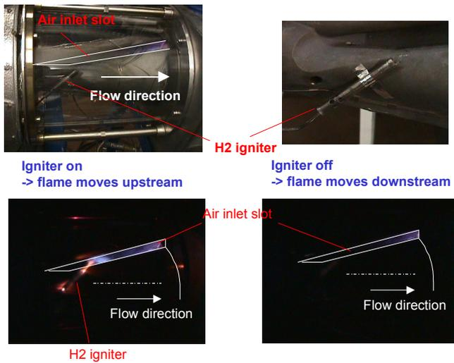
**Fig. 16** Forced atmospheric hydrogen flashback test
