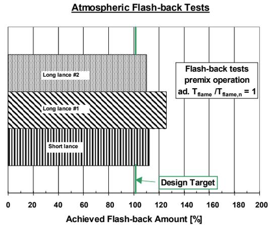
**Fig. 15** Atmospheric hydrogen flashback tests
