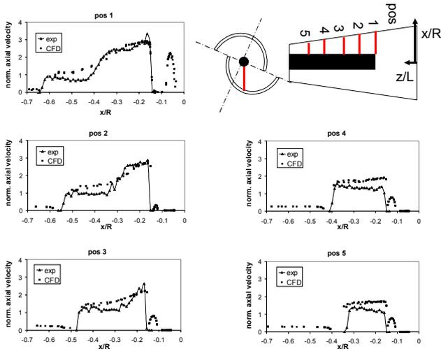
**Fig. 12** CFD calculations of the axial flow field around the extended lance compared with water tunnel measurements.
