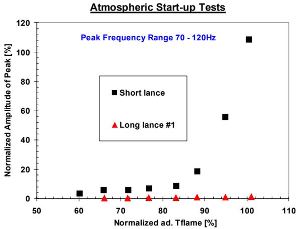
Fig. 9 Atmospheric startup tests. Flame temperature variation.
