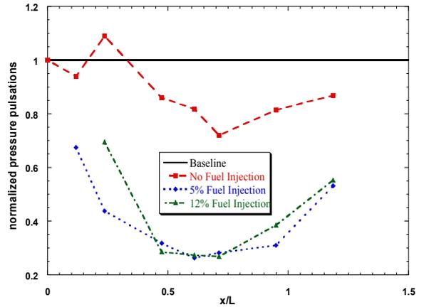
**Fig. 6** Suppression of pressure pulsations for different lance lengths
