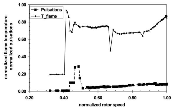
**Fig. 18** Reduced pulsations in a startup test in the test engine using the long lance.
