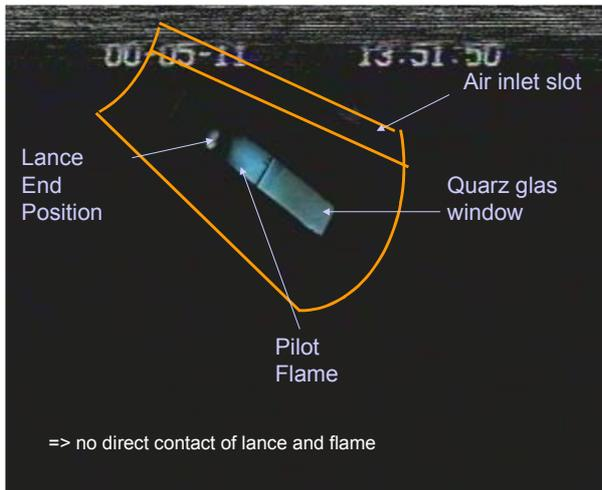
**Fig. 14** Video image of combustion in the high pressure rig, indicating that the flame is stabilized downstream of the extended lance
