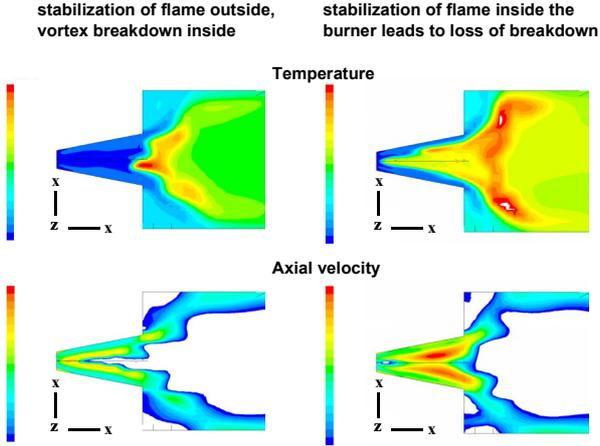
Fig. 4 CFD simulation of the pilot instability
