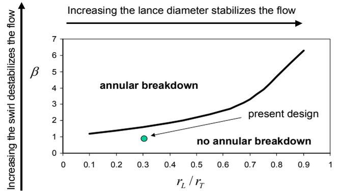
Fig. 11 Critical swirl for a single vortex ( $w_1 = u_1$ ). Present design shown to be in stable region.
