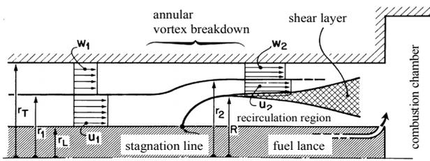
Fig. 10 Schematic of the configuration used for annular breakdown analysis.
