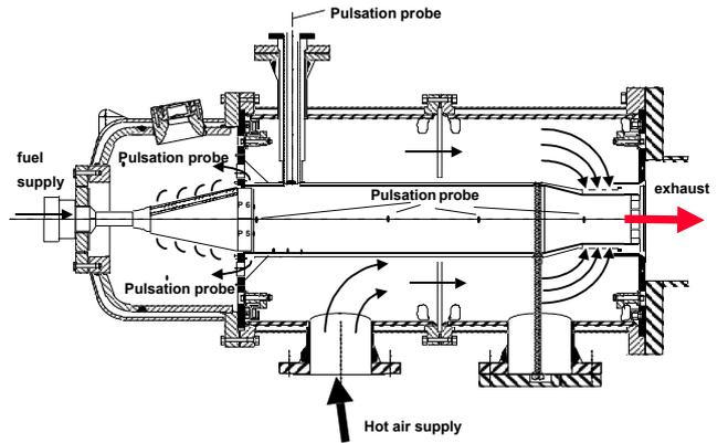
**Fig. 2** Schematic of the high pressure test facility
