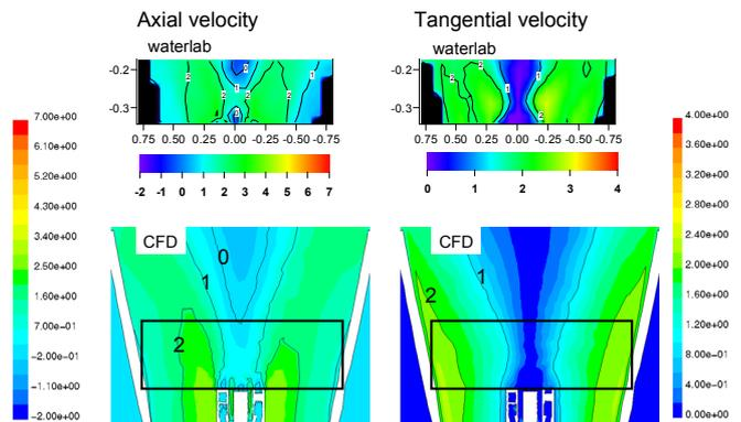
**Fig. 13** CFD calculations of the flow field downstream of the lance compared with water tunnel measurements.
