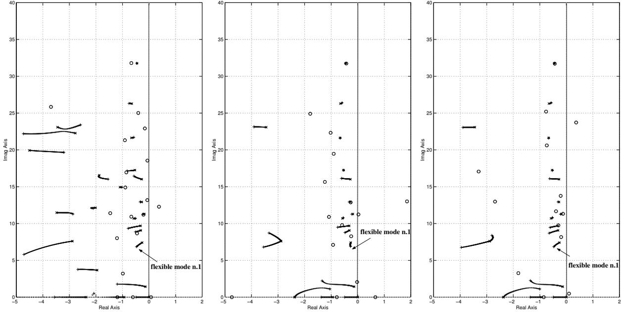
**Fig. 3** Root loci at  $m_1$  for the initial  $\mathcal{H}_2$  controller (on the left), the intermediate (in the middle) and the final modal dynamic controller  $K_0(s)$  (on the right)
