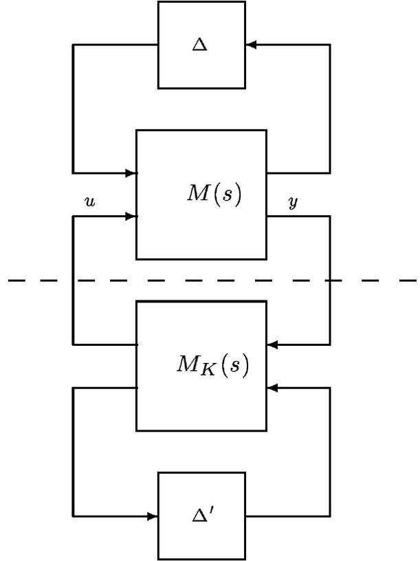
**Fig. 1** LFT-formulation of the system controlled by a dynamic self-scheduled output feedback
