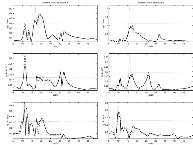
**Fig. 4** Frequency domain responses of lateral acceleration  $n_{y,i}$  of the open-loop (dotted lines), the initial  $\mathcal{H}_2$  controller (dash-dotted lines) and the equivalent modal dynamic controller  $K_0(s)$  (solid lines) for the two models  $m_1$  (left) and  $m_6$  (right)
