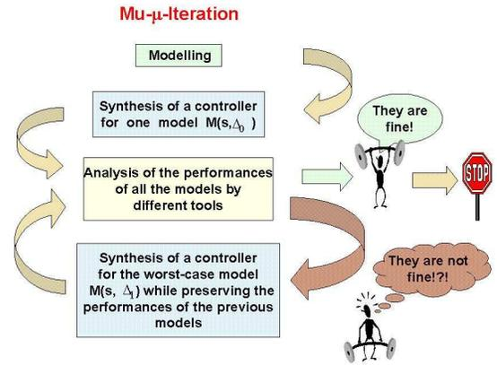
Fig. 2 The multi-model (Mu- $\mu$ )-Iteration
