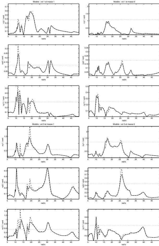
**Fig. 5** Frequency domain responses of lateral acceleration  $n_{y,i}$  of the initial  $\mathcal{H}_2$  controller (dashed line) and the dynamic modal self-scheduled controller  $K_{sched}(s, \delta V)$  (solid line) for the two models  $m_1$  and  $m_6$  at speeds  $V_1$  and  $V_3$
