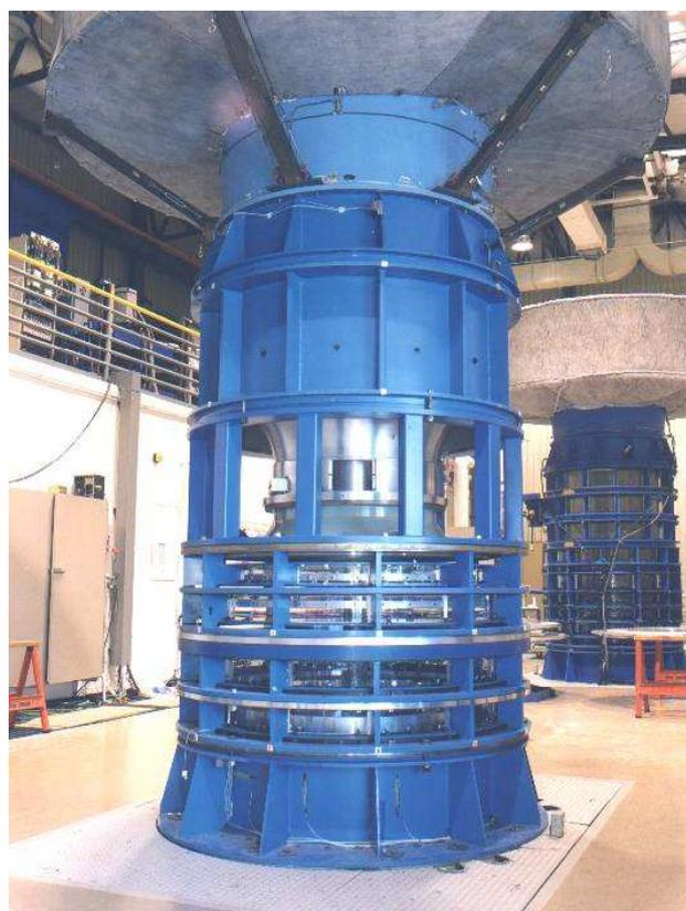
**Fig. 1** The Low Speed Research Turbine (LSRT) in sloped end-wall configuration (Low Speed Research Compressor in background)
